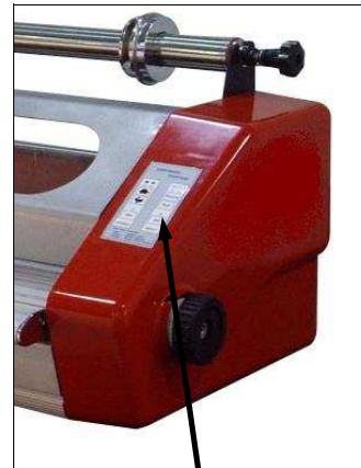
Figure 3 Location of Control Panel
