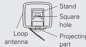
**2** Insert the projecting part into the square hole in the stand.
