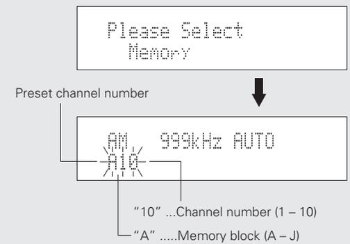
**3** While the preset channel number is flashing, turn **<TUNING/PRESET>** and select the desired preset channel number.
