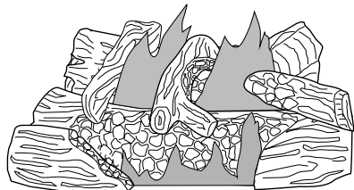
Figure 51 - Typical Flame Pattern
