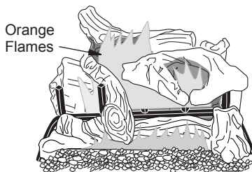
Figure 24 - Incorrect Burner Flame Pattern
