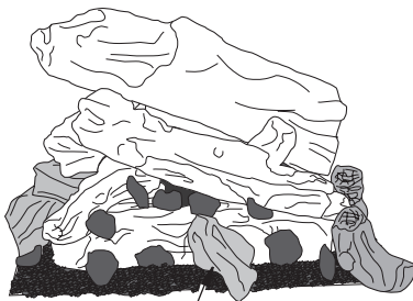
Figure 31 - Installing Scrap Log Pieces
