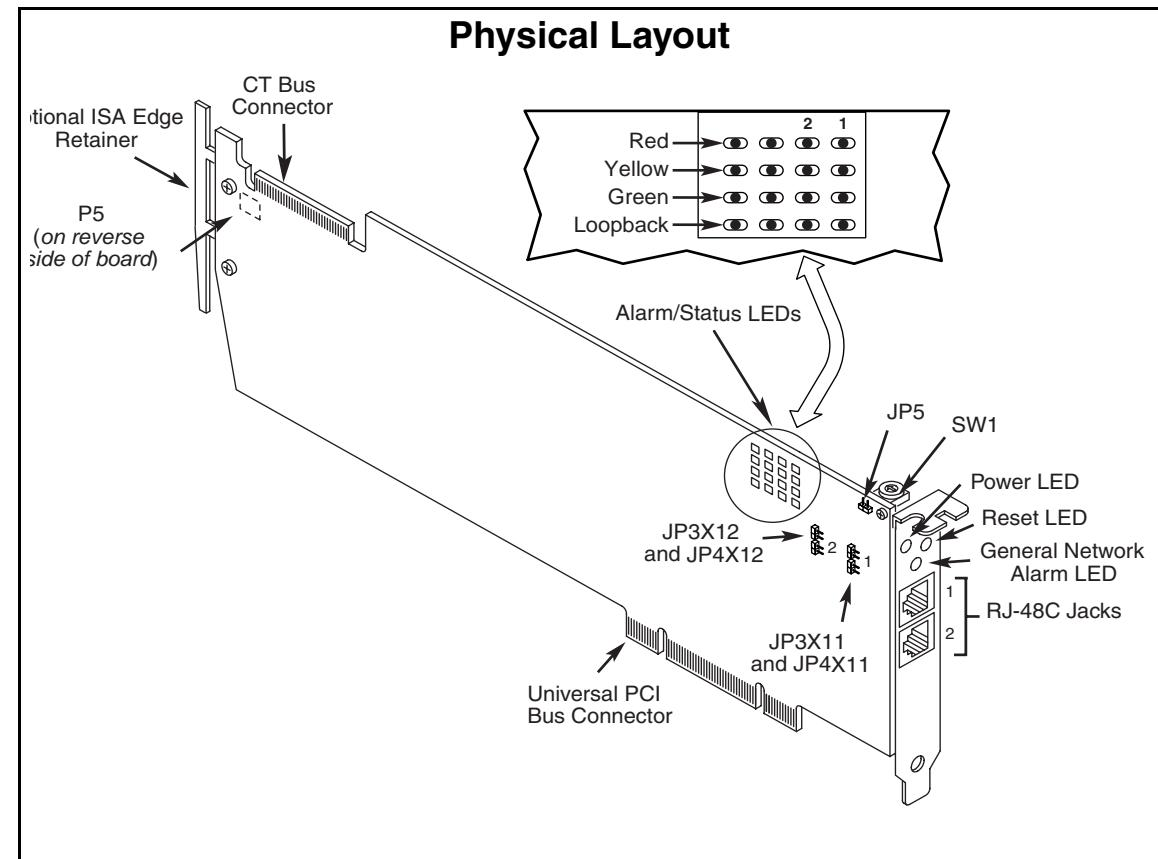
**CT Bus Connector:** Connector to CT Bus.
