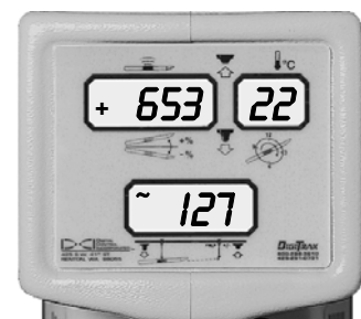
Locating Mode Showing Signal Strength, Transmitter Temperature, and Predicted Depth
