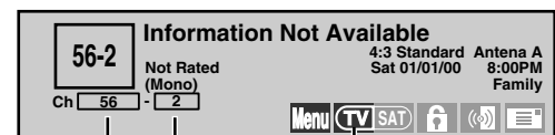
Primary channel entry box Subchannel entry box Highlighted to indicate TV mode
