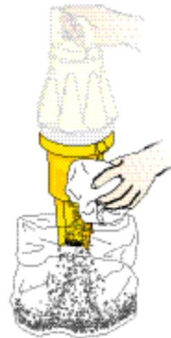
UK. Press catch 3 to release bin. Remove fine dust with a cloth or brush.
