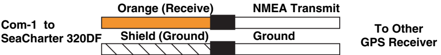
Com-1 wiring to receive NMEA position information from some other GPS receiver.
