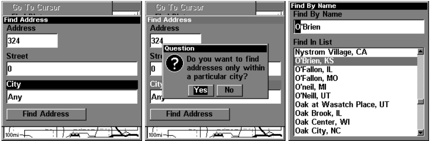
Find City field, left, Search in particular city only option, center; Find City by name, right.
