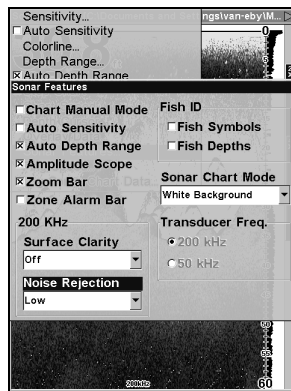
Sonar Menu with Sonar Features selected (left). In the Sonar Features menu, Noise Rejection is selected with ASP in the default low setting (right).
