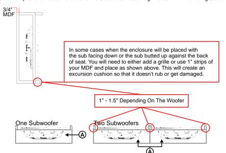
SWS subwoofers will handle crazy amounts of power in any of the recommended enclosures, minimum or maximum. The compact enclosures are best for use in limited-space applications. The larger recommended enclosures will deliver a bit more bass at the lowest frequencies ranges.
