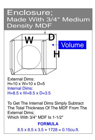
**CAUTION:** In some cases when the enclosure will be placed with the sub facing down or the sub butted up against the back of seat (like the illustration). You will need to either add a grille or use 1" strips of your MDF and place as shown above. This will create an excursion cushion so that it doesn't rub or get damaged.
