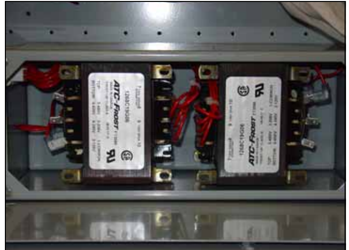
Figure 16. North American Market Voltage Selection Terminals (Shown Connected to the 120 Vac Taps).
