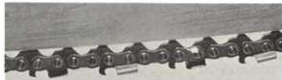
B. Chain is improperly tensioned
