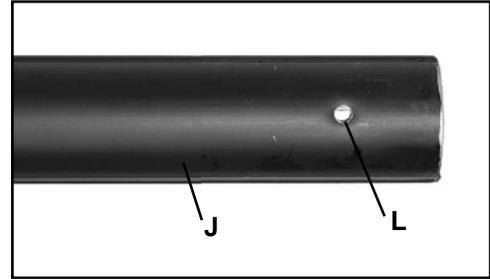
9. Align ridges on aluminum extension housing (J) with seams in cutting attachment and slide cutting attachment onto extension housing. Remove locator screw (B) to align locating hole in cutting attachment with locating hole (L) in aluminum extension housing.
