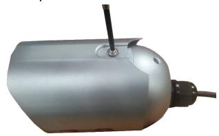
8. Secure the wall mouting metal bracket on the wall then secure the bullet camera on the bracket. There ae two spots available.
