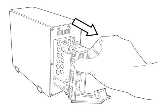
4. Use your finger to remove white bracket in HDD enclosure, as instructed by the arrows.
