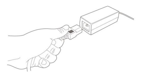
10. Insert the AC adapter's power plug into NVR's power socket.
