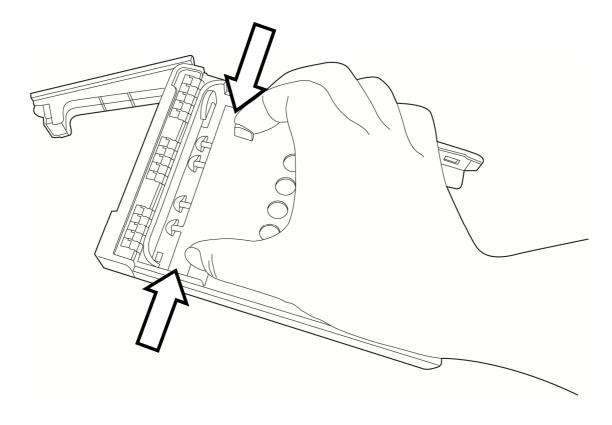
5. Put a 3.5" SATA HDD in the HDD enclosure, as instructed. HDD's SATA connector should be located at left.
