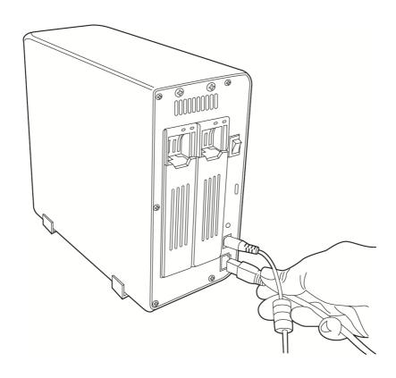
12. Switch the power switch of NVR on. The 'POWER' LED on the front panel of NVR should light up now. If not, please recheck step 7 to 9 and make sure the power outlet you are connecting to is properly working.
