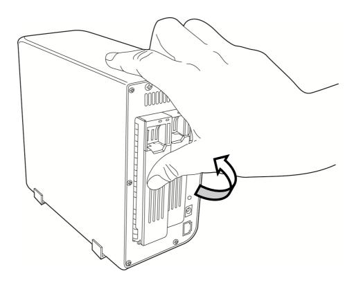
Note: Do not pull the hard drive out when the NVR is powered on, or data stored on the hard drive will be damaged.
