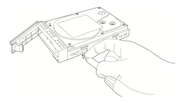
7. Press the top of HDD enclosure and fully push it back into NVR, as instructed (do not press white lever back now, and it should remain in open position in this step).
