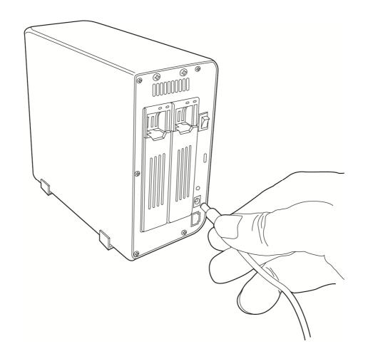
11. Insert the Ethernet cable into NVR's Ethernet socket. The other end of Ethernet cable should connect to your local network's hub or switch.
