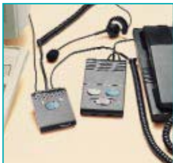
The SeleCT system easily connects your headset to both your telephone and computer, so you can move from one to the other with the flick of a switch. A 6-foot cord with standard 3.5 mm phono jacks is included.
