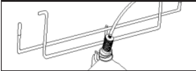
Figure 15 — Insert Filter into Container
