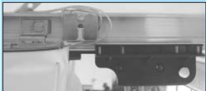
FIG. 7-4 Align "OPEN" limit switch.
