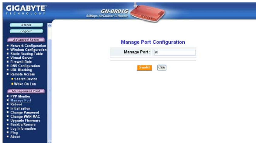
Figure 7-2 – Manage Port Config screen
