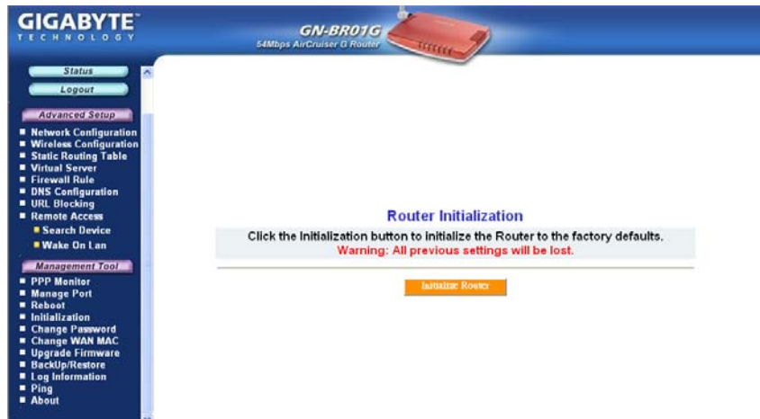
Figure 7-4 – Router Init Screen
