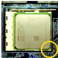
Fig.2 Pin 1 location on the socket and processor. Gently place the CPU into position making sure that the CPU pins fit perfectly into their holes. Once the CPU is positioned into its socket, place one finger down on the middle of the CPU and gently press the metal lever back into its original position.
