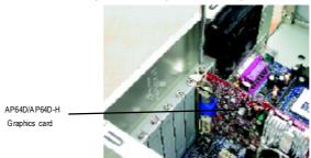
6. Plug the display cable into your card; then turn on the computer and monitor. If your Graphics card came with a DVI connector, you can connect a flat panel display to the appropriate connector, as shown below...
