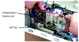
5. Replace the screw to fasten the card in place, and replace the computer cover.
