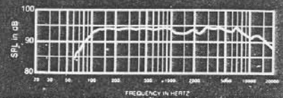
FIGURE 1 — Axial Frequency Response 4 volts/10 feet
