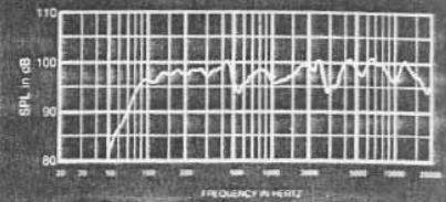
FIGURE 1 Axial Frequency Response, 4-Volts/10 Feet
