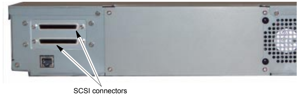
Figure 2-8 SCSI connectors on the back of the autoloader
