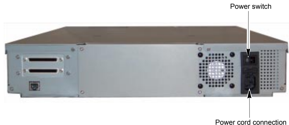
Figure 2-11 Location of the power switch and power connector
