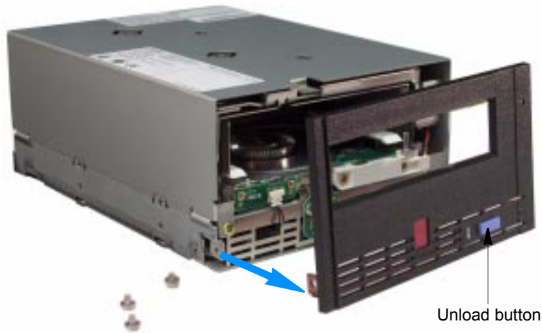
Figure 7-7 Removing the faceplate from the tape drive chassis
