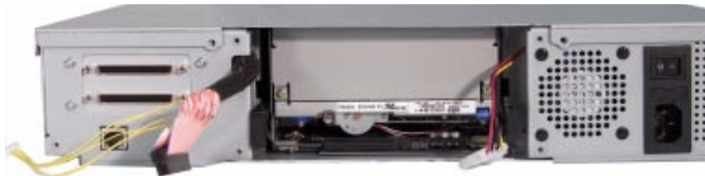
Figure 7-11 Full height tape drive installation
