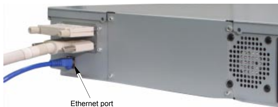
Figure 2-10 Connecting the autoloader to an Ethernet network
