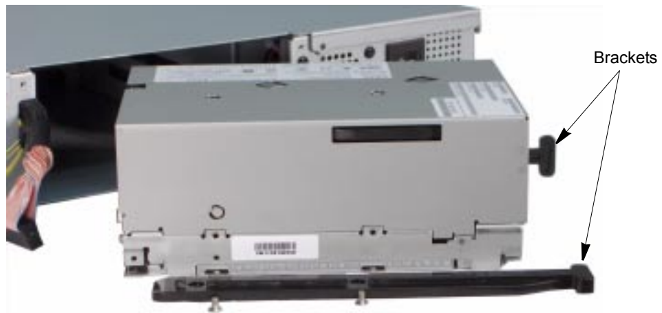
Figure 7-5 Removing the brackets from the tape drive
