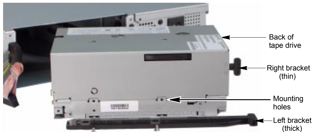
Figure 7-9 Attaching the brackets to a full height tape drive
