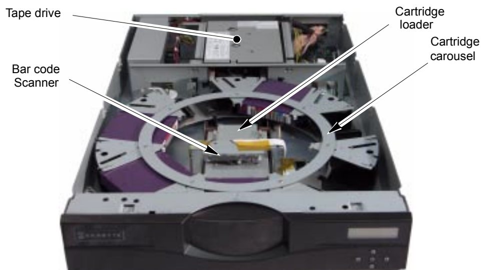
Figure 1-3 Magnum 1x7 LTO Autoloader internal components
