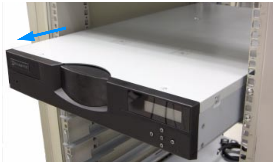
Figure 9-2 Removing the autoloader from the rack
