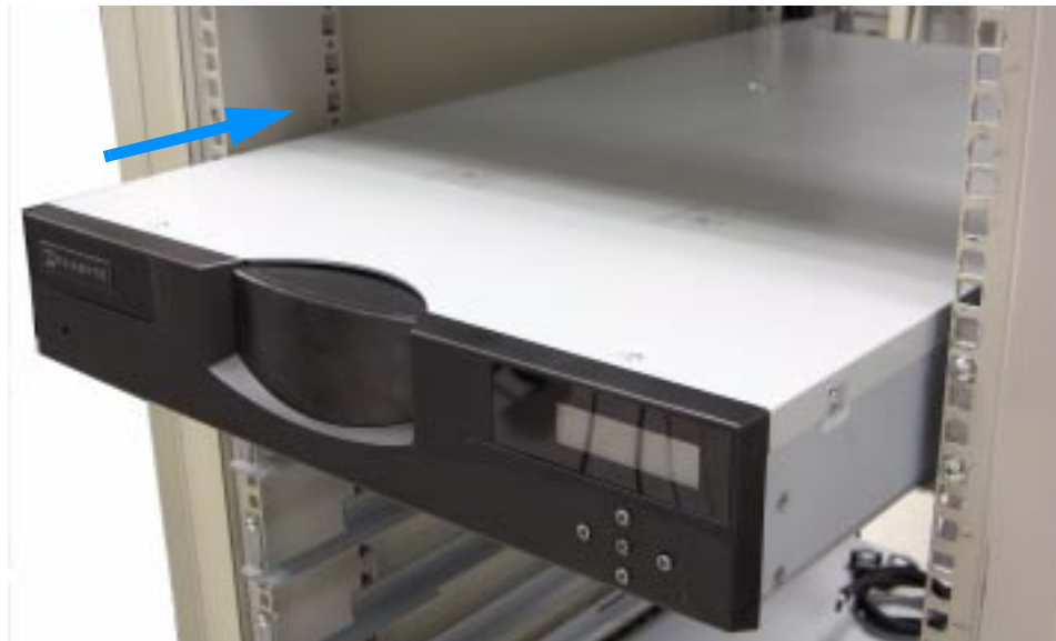
Figure 2-6 Placing the autoloader on the rails
