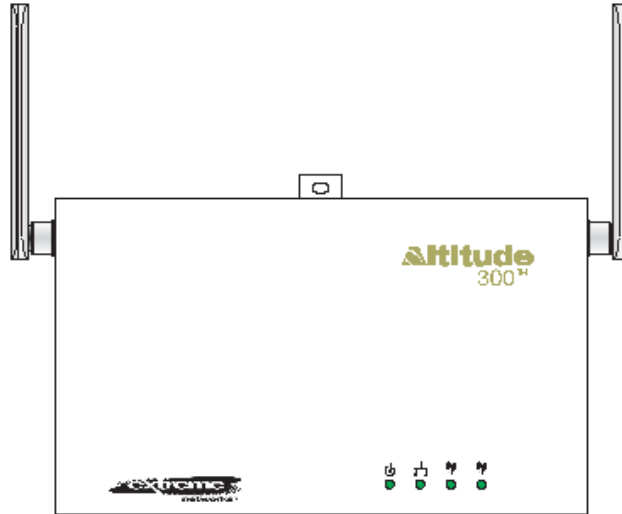
Figure 3: Altitude 300-2™ LED Indicators, without Plastic Cover LED Indicator Functions
