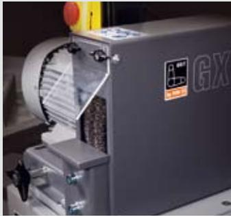
Independent of the GX program, the GXE machine utilizes durable steel brushes for deburring steel and stainless steel workpieces. Available with optional pedestal base and steel or stainless steel brushes.
