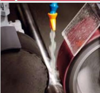
Add-on module for finishing and polishing applications on round, ferrous and non-ferrous stock – from rough grinding to mirror polish.
