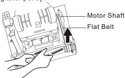
Place a new flat belt onto the motor shaft and pulley.
