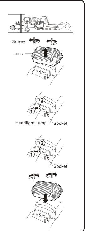
**Caution:** Be sure to turn the ON/OFF switch to the "OFF" position and disconnect the power cord from the wall outlet before replacing any of the parts below.
