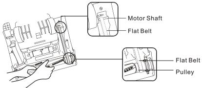
4 Place the agitator assembly into the grooves in the nozzle head, making sure that the new flat belt slides securely into the guide.
