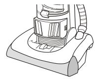
2 Re-tighten the screw using a Philips screwdriver and slide the latch in the direction indicated by the arrow.
