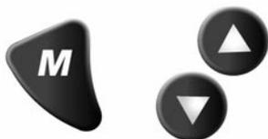
that control the functions available. The “Mode” button is used to change the function of the LCD display and to access submenus and adjustable settings.
