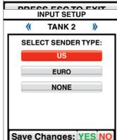
**TANK 2** – Select the type of level sender connected to Pin 6 on HN0605\*. If nothing is connected, select “NONE”.
