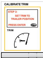
**Step 3:** Set your engine to the top of its trailer / full-up position, then press **ENTER**.
