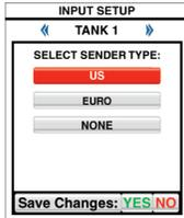
**TANK 1** – Select the type of level sender connected to Pin 5 on HN0605\*. If nothing is connected, select “NONE”.
