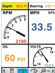
quadrant is highlighted, press **ENTER**. A list of options will appear in the center of the screen. Use the up or down arrows on the navigation pad to highlight the desired information to be displayed, then press **ENTER**. The highlighted quadrant will change to the selected display.
