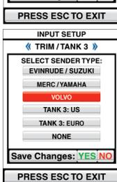
**TRIM / TANK 3** – Choose the type of analog trim sender or level sender connected to Pin 7 on HN0605\*. If nothing is connected, select “NONE”.
