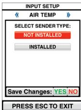
**AIR TEMP** – Select “INSTALLED” if an analog Air Temp sender is connected to Pin 9 on HN0605\*. If an air temp sender is not connected, select “NOT INSTALLED”
