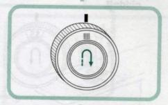
针距选择旋钮转到"#"处,送料牙工作时, 齿面低于针板上平面,不起送料作用。 Embroidering and darning are best carried out with the feed machanism disengaged. This is done by setting the stitch length dial at, which drops the feed and allows the material to be moved freely under the needle.
