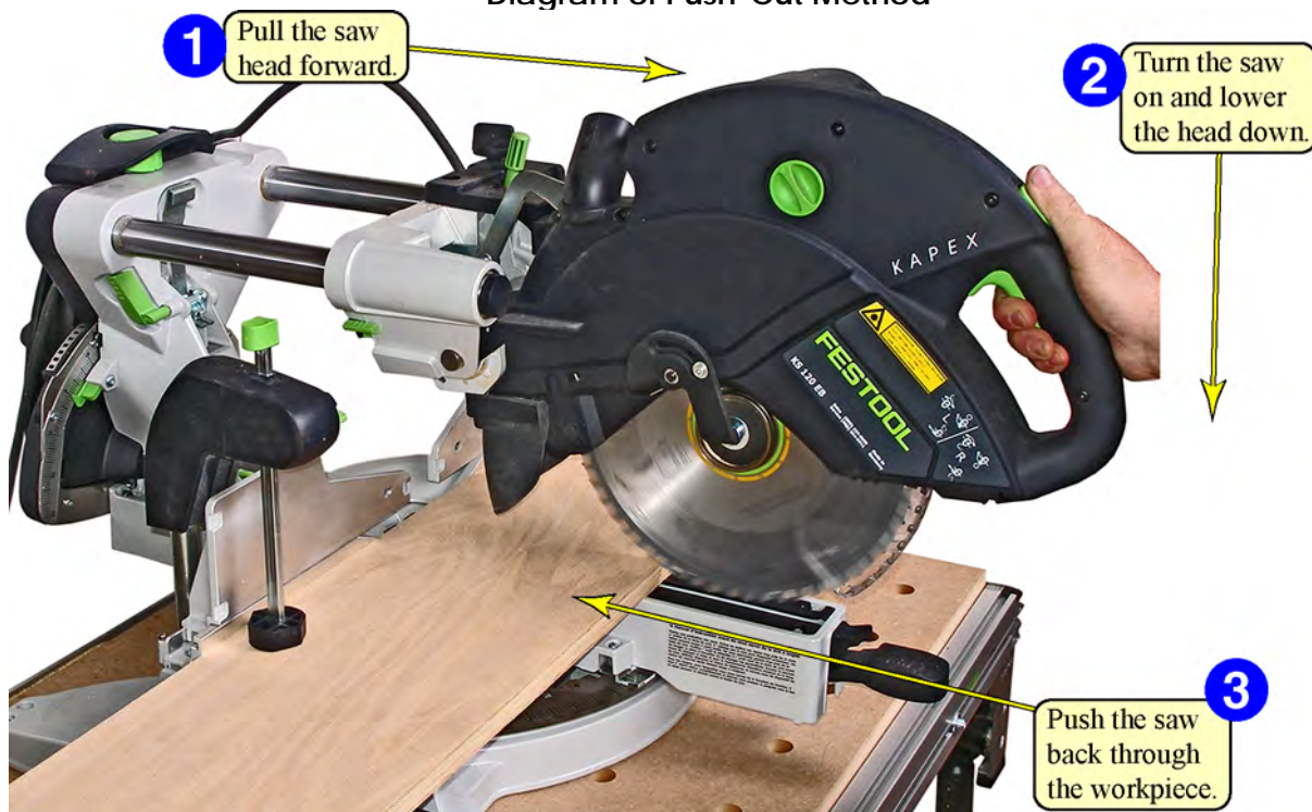
Diagram of Push-Cut Method
