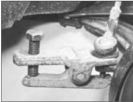
2.2 Disconnecting a tie-rod end balljoint
