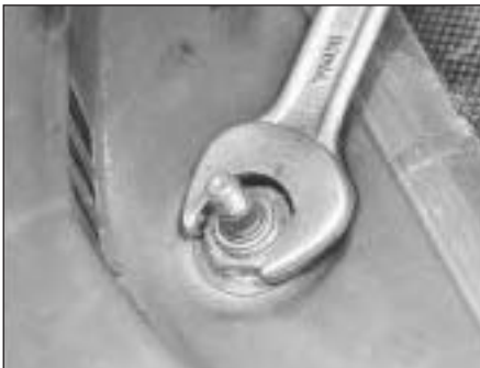
15.95 Unscrewing the wiper pivot nut
