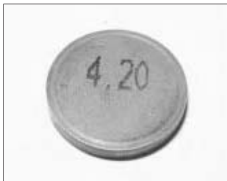
2B.25A Valve clearance shim showing thickness mark
