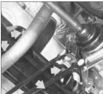
Fig. 11.6 Steering rack mounting bolts (Sec 7)
