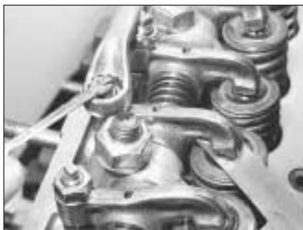
5.7 Adjusting a valve clearance
