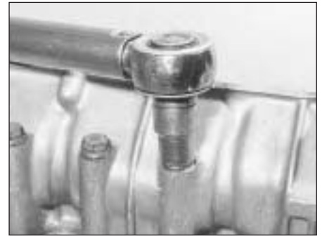
27.18 Tightening a camshaft carrier bolt
