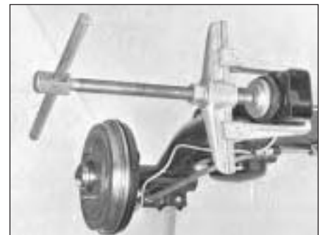
Fig. 11.10 Method of renewing trailing arm bush (Sec 10)
