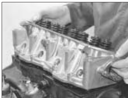
7B.120A Lower the cylinder head onto the block . . .
