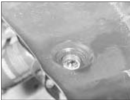
2.6 Engine sump drain plug
