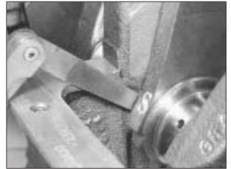
20.10 Checking crankshaft end float
