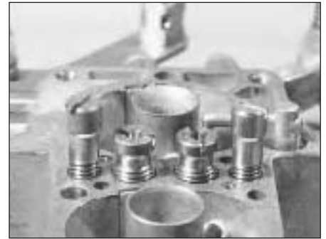
9B.41 Jets on the Weber 30/32 DMTE carburettor (top cover removed)
