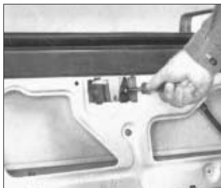
Fig. 12.6 Door glass mounting screw (Sec 12)
