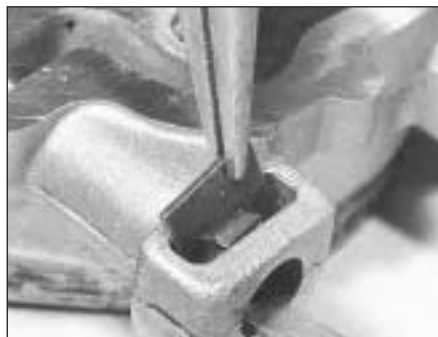
5B.72A Removing the oil pump relief valve keeper plate
