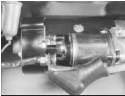
8.2 Starter motor connections
