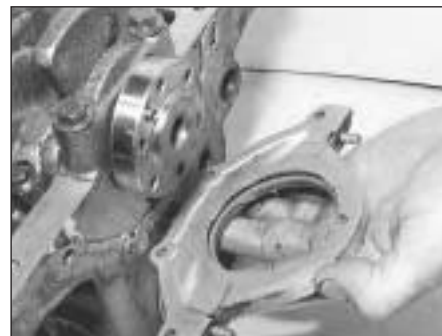
5D.9 Fitting crankshaft rear oil seal retainer
