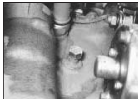
8C.9 Cylinder block drain plug
