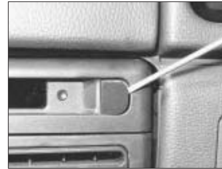
15.62 Prise free the trim covers for access to retaining screws . . .
