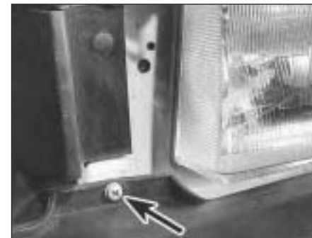
17.24 Front bumper upper mounting screw (arrowed)
