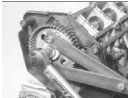
7B.48 Tightening the crankshaft sprocket bolt
