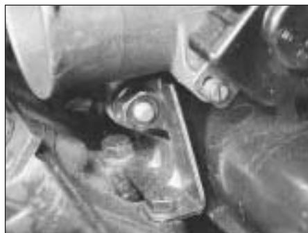
9C.78 Throttle valve housing support bracket
