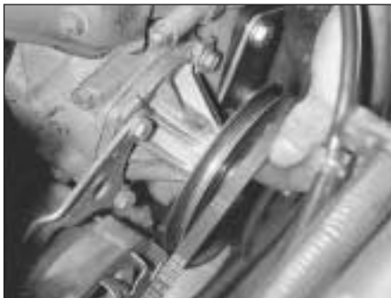
8C.52 Fitting a new coolant pump/alternator drivebelt around the pulleys
