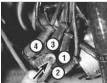
10.72 HT lead connecting sequence on the 1301 cc Turbo ie engine
