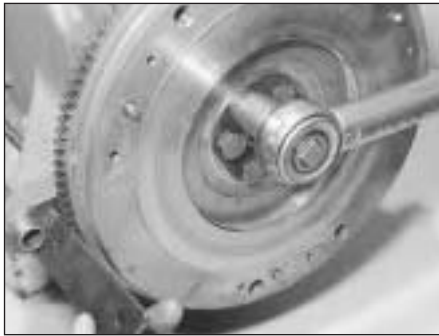
42.19 Tightening flywheel bolts
