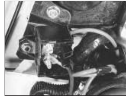
15.26B Battery lead terminal block on the 1301 cc Turbo ie model
