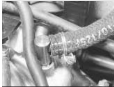
44.21B Brake servo hose at manifold
