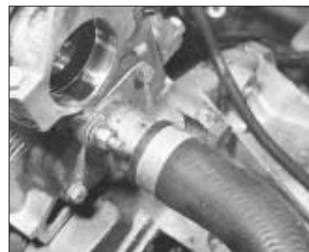
8A.6 The thermostat housing (shown with distributor removal) on the 999 cc engine
