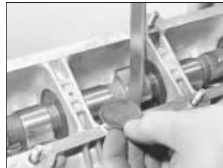
7B.15 Removing a shim from a cam follower
