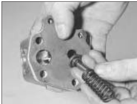
7B.180A Locate pressure relief valve and spring on the intermediate plate
