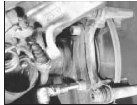
14B.42 Unscrewing a rear caliper bracket bolt
