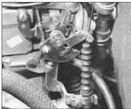
5C.12 Choke cable connection at carburettor
