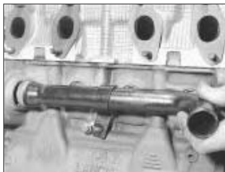
5D.30 Coolant distribution pipe
