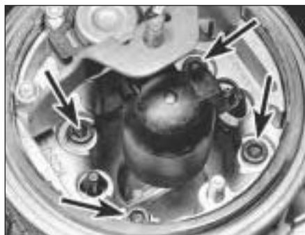
9D.44 Injector unit retaining screws (arrowed)
