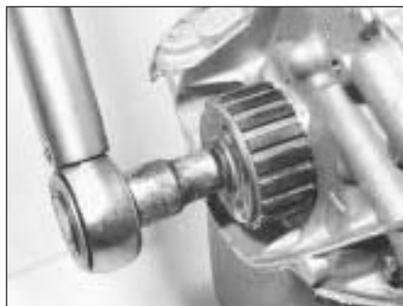
5D.16B Tightening the crankshaft sprocket bolt
