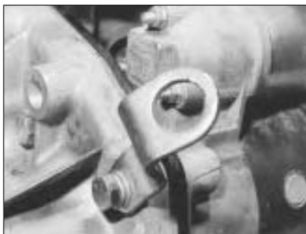
5D.38 Lifting eye on flywheel housing flange
