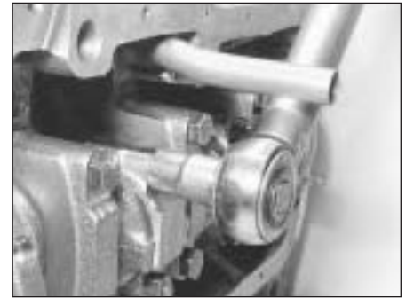
32.16 Tightening a big-end cap nut
