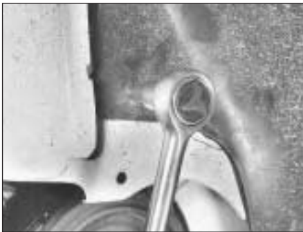
10.4A Unscrewing wing shield screw
