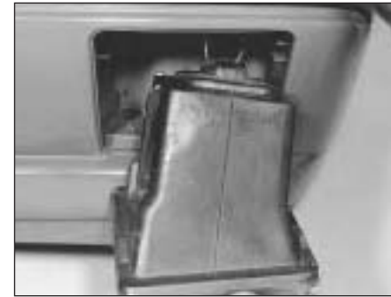
15.37B . . . and withdraw the front fog lamp unit . . .
