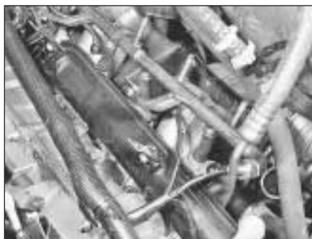
9C.81B Fuel injector cooling air duct refitting
