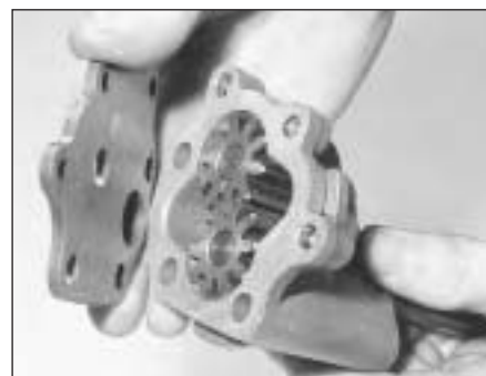
7B.179 Refitting the intermediate plate
