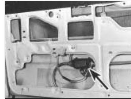
17.34C Door interior showing electric window motor (arrowed)
