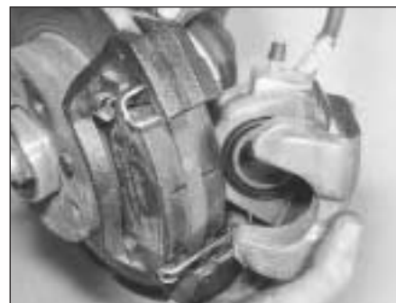
3.4 Removing the caliper unit
