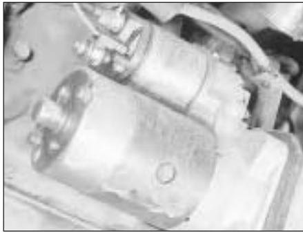
15.23B Starter motor and wiring connections on the 1372 cc ie engine
