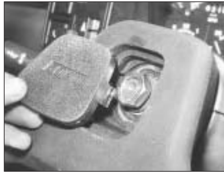
4.2 Removing steering wheel hub plate
