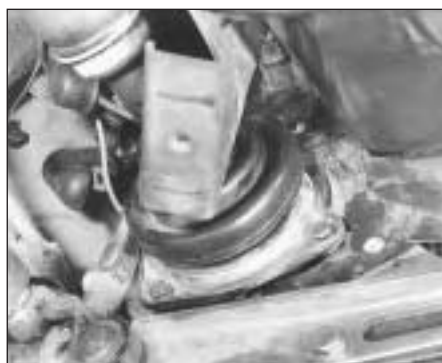
5C.24C Gearchange rod support bracket
