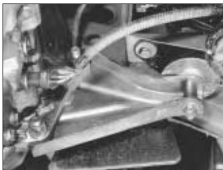
7C.36C Transmission front mounting
