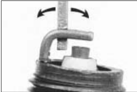
Adjusting spark plug gap
