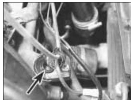
6B.22 Distributor drive hole cover plate (arrowed)
