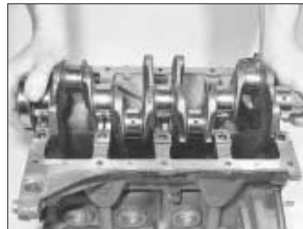
5D.4 Fitting the crankshaft
