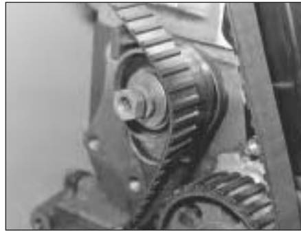
28.8 Slipping timing belt onto tensioner pulley
