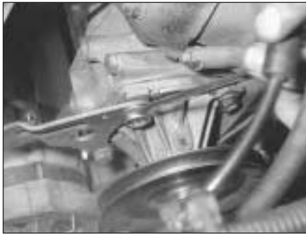
8C.40 Coolant pump/alternator bracket bolt removal
