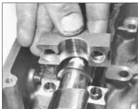
5B.23D Camshaft bearing cap showing short and long positioning dowels for correct fitting
