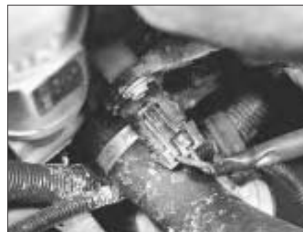
8C.21B Cooling fan switch wiring connector
