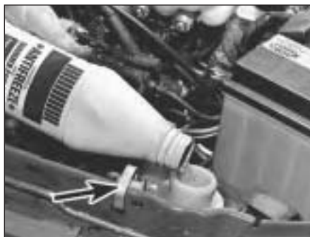
8C.28 Topping up the radiator coolant level on the 1372 cc ie engine. Note orientation of radiator retaining clip (arrowed)
