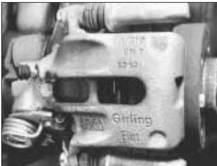
14B.23 Rear brake pad inspection aperture
