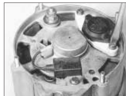
15.16A Extracting the alternator brush holder screw
