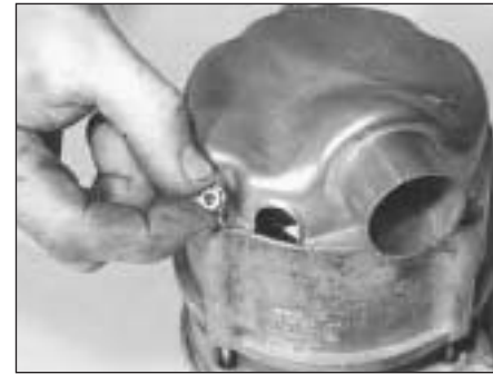
15.12B Alternator rear cover and fixing nut
