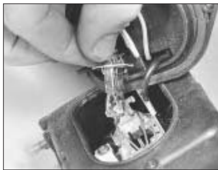
15.39 . . . detach the wires, extract the bulb
