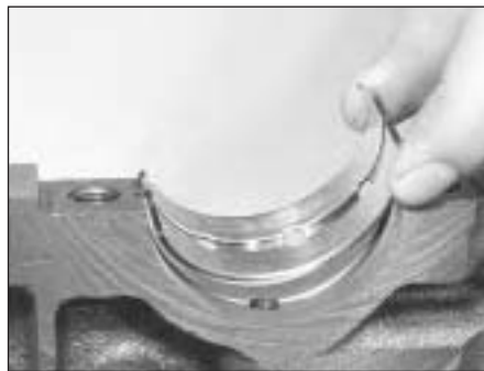
20.1 Fitting a main bearing shell
