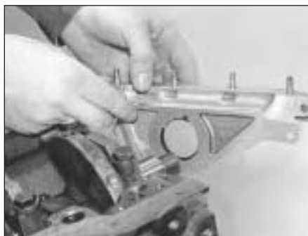
7B.141A Refit the crankshaft front oil seal housing . . .
