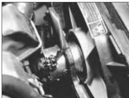
8C.21A Cooling fan and wiring connector
