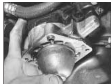
15.23A Starter motor removal from the 1301 cc Turbo ie engine
