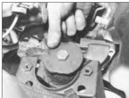
5C.31A Right-hand engine mounting disconnected
