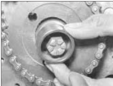
6.15 Fitting fuel pump drive cam and sprocket bolt
