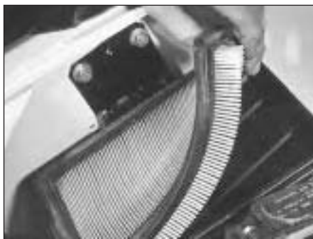
9C.27B Removing the air cleaner element
