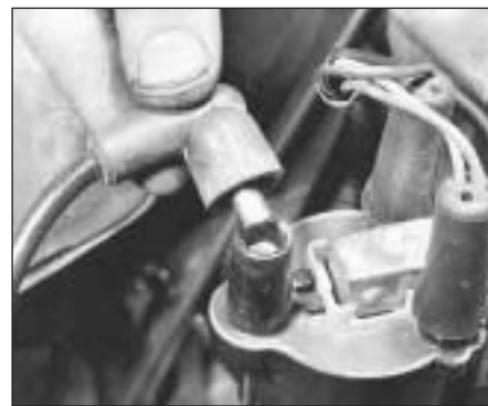
5C.15 Ignition coil HT lead connection
