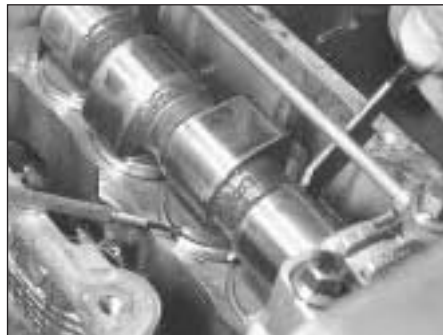
5B.1B Using a modified C-spanner and screwdriver to remove a shim
