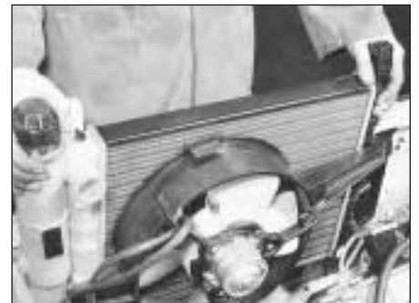
7.4B Removing radiator/fan assembly
