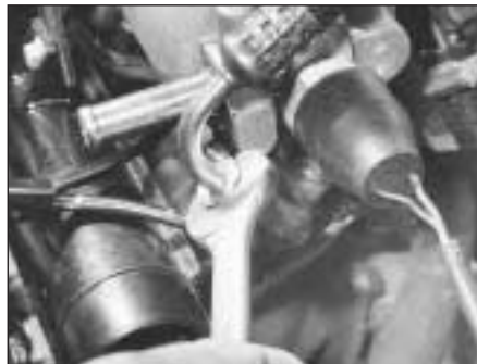
9C.75 Disconnecting the fuel delivery hose union
