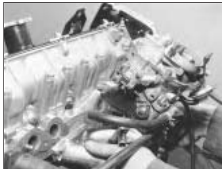
19.4C Fitting intake manifold complete with carburettor
