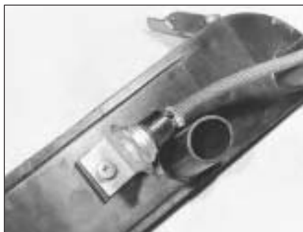
9C.79 Fan thermostatic switch on underside of injector cooling air duct (duct removed for clarity)
