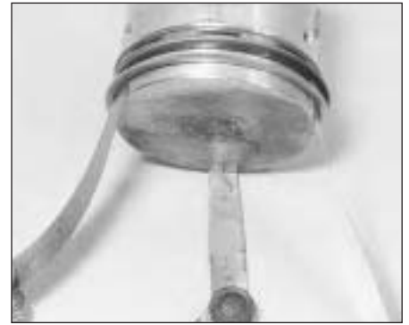
18.20 Using feeler blades to fit piston rings
