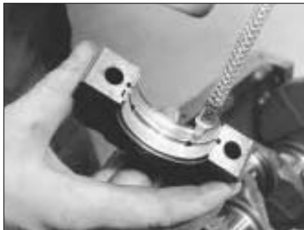
7D.9 . . . and lubricate the shells
