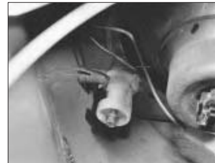
15.29 Headlamp beam adjuster on the 999 cc Turbo ie model
