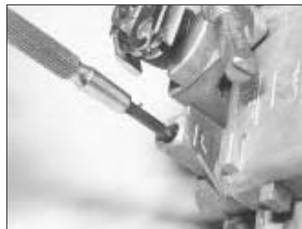
9B.9 Mixture adjustment - Weber 32 TLF carburettor
