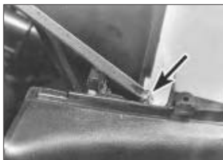
21.3 Removing instrument panel screw
