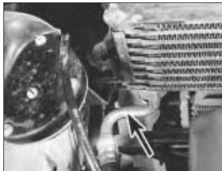
6B.24A Oil cooler pipe connection (arrowed)
