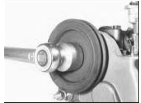
20.23 Tightening crankshaft pulley nut
