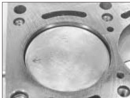
5B.96 Piston directional arrow
