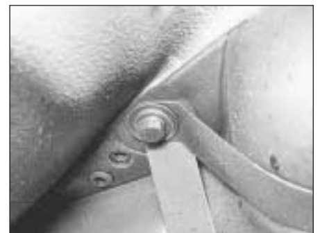
5.4 Fuel tank mounting straps
