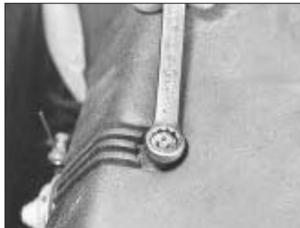
9A.6 Air cleaner casing nut on the 999 cc model
