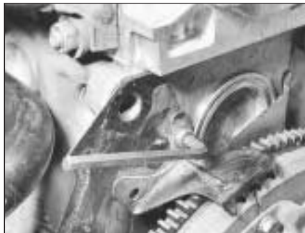
5C.62 Unscrewing socket-head screw from timing index plate
