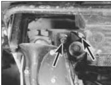
6B.25 Oil cooler mounting bolts (arrowed)
