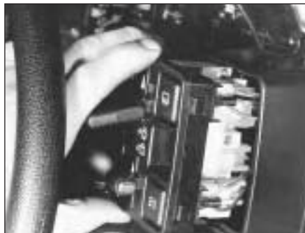
15.54A Switch block withdrawal on the 1301 cc Turbo ie model
