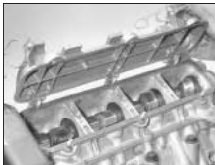
7B.89B . . . and refit the camshaft cover
