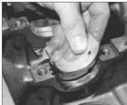
7D.6A No. 3 main bearing shell is plain . . .
