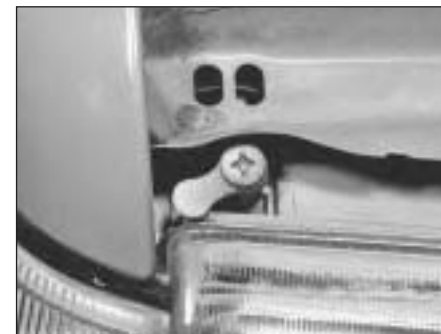
15.31B Headlamp vertical beam alignment adjuster screw on a 1372 cc ie model. Note the load compensator lever which is set in the "O" (normal load) setting position
