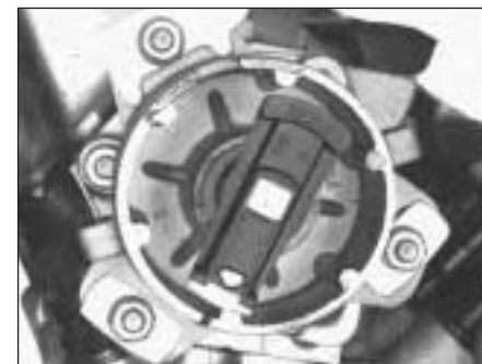
Fig. 13.78 Rotor aligned with distributor body rim mark - Microplex ignition system (Sec 10)
