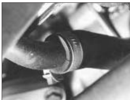
9F.20 Turbocharger oil return pipe at sump
