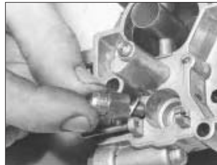
9B.26B Fuel inlet valve needle removal from the Weber 32 TLF carburettor
