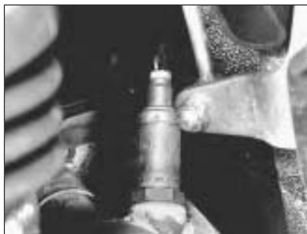
9D.69 Lambda sensor in exhaust downpipe
