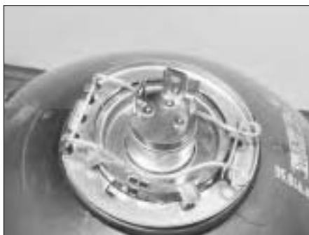
16.2A Headlamp bulbholder spring clips
