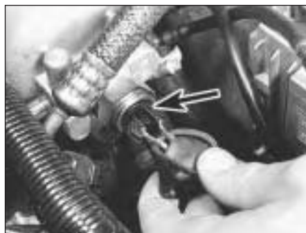
9F.5 Maximum air pressure switch (arrowed)
