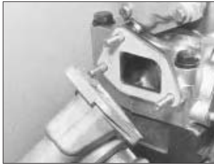
4.4 Fitting thermostat housing (1116 cc engine)
