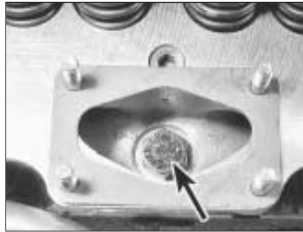
7.24A Cylinder head bolt in intake manifold
