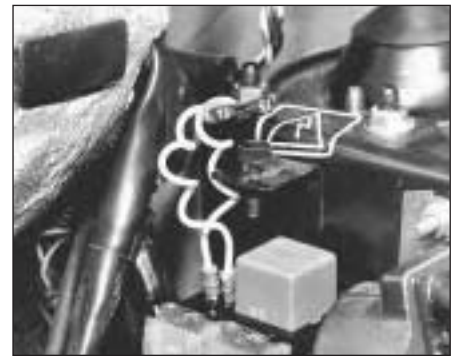
9D.30 Test lead connected to relay terminals 30 and 87
