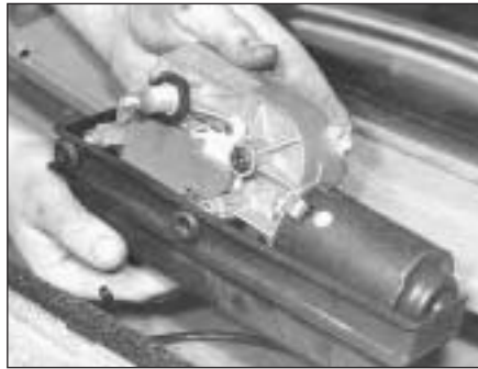
15.98B . . . separate the wiper motor from its cover . . .
