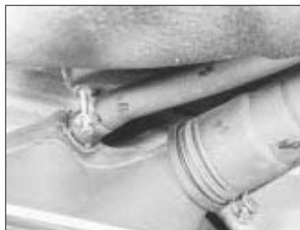
5.3 Fuel tank filler and vent hoses
