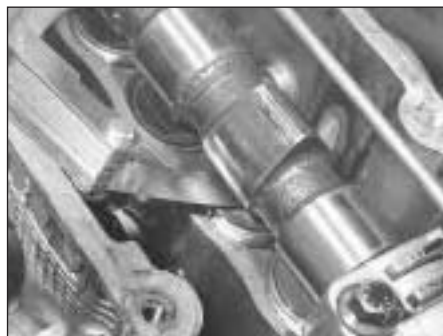
5B.1A Checking a valve clearance
