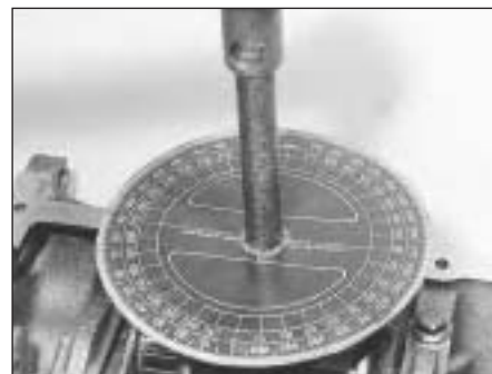
5D.7B Angle-tightening a main bearing cap bolt
