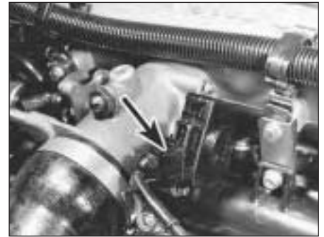
9C.90 Throttle position switch (wiring plug arrowed)
