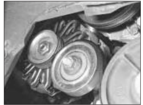
8C.49 Alternator/water pump drivebelt and tensioner viewed from the right-hand wheel arch
