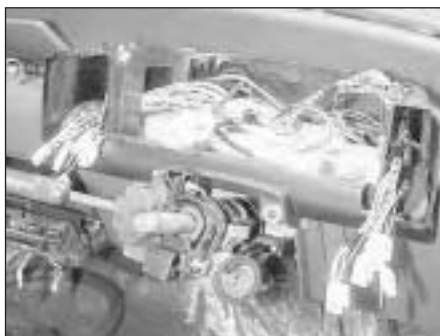
21.5 Instrument panel and steering wheel removed
