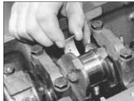
7B.195 Assemble the shell bearing to the connecting rod . . .
