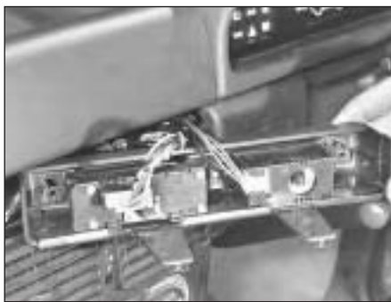
15.63 . . . and withdraw the auxiliary control panel
