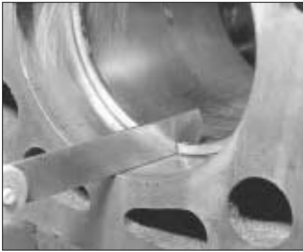
18.24B Checking piston ring end gap
