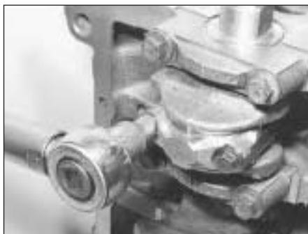
5B.99 Tightening a big-end cap bolt
