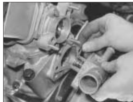
8C.31 Thermostat unit removal on the 1372 cc ie engine (distributor removed for clarity)
