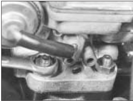
9B.37F Unscrewing a carburettor fixing nut
