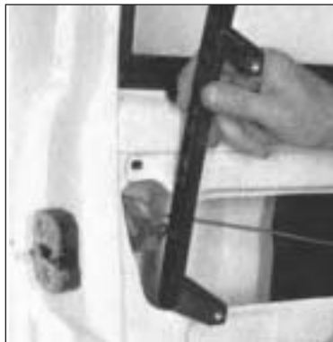
Fig. 12.13 Removing glass guide channel (Sec 12)
