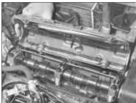
5B.20B Removing the camshaft cover
