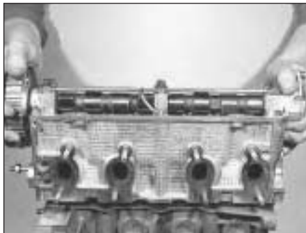
5B.51 Fitting the cylinder head
