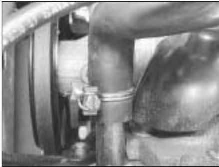
44.21A Heater hose at manifold
