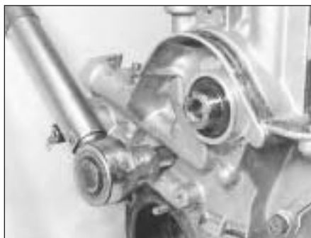
5D.12B Tightening an oil pump bolt
