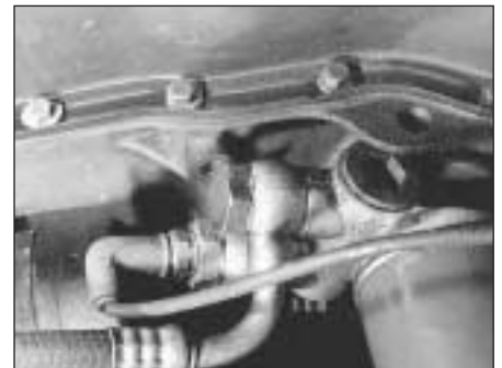
6B.24B Connections at oil filter cartridge mounting base
