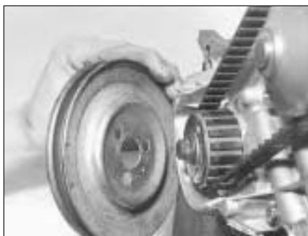
5D.22 Crankshaft pulley installation
