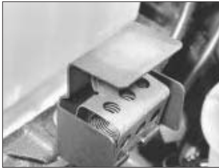
15.34 Headlamp dim-dip transformer
