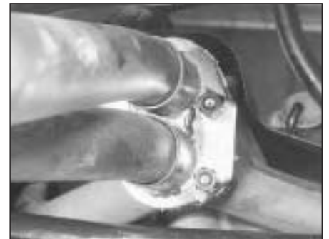
44.15 Exhaust downpipe flange nuts
