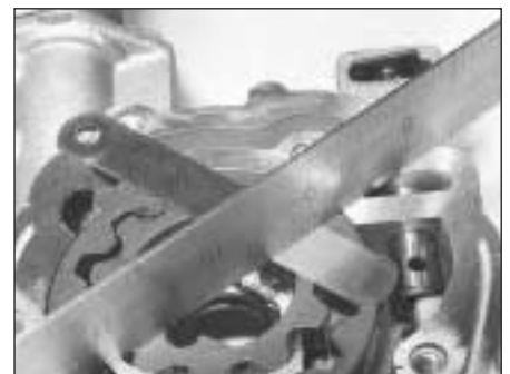
5B.74B Checking the oil pump gear endfloat
