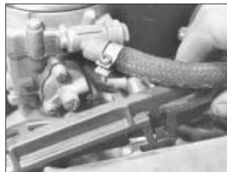
5B.20A Camshaft cover HT lead clip
