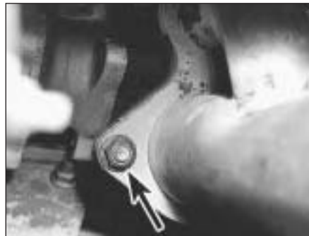
9F.16A Turbocharger-to-exhaust flange nut (arrowed)
