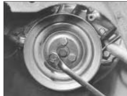
5B.7 Unscrewing the crankshaft pulley bolts
