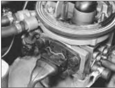
7C.20 Fuel injector wiring connection
