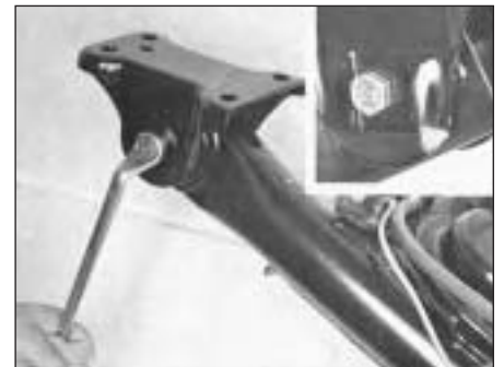
Fig. 11.9 Removing trailing arm pivot bolt (Sec 10)
