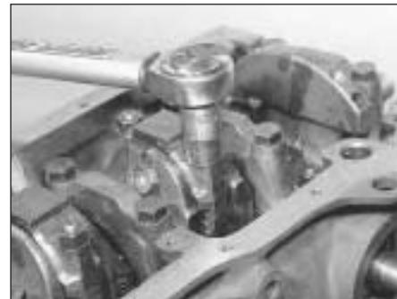
7B.197B . . . and tighten the nuts to the specified torque
