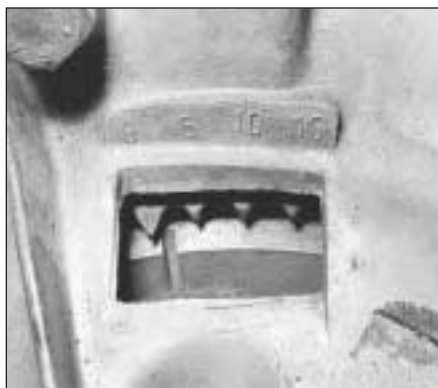
10.2A Flywheel timing marks (999 cc engine)
