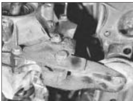
5C.26 Left-hand rear (lower) transmission mounting disconnected
