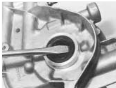
5B.77A Removing the oil pump seal
