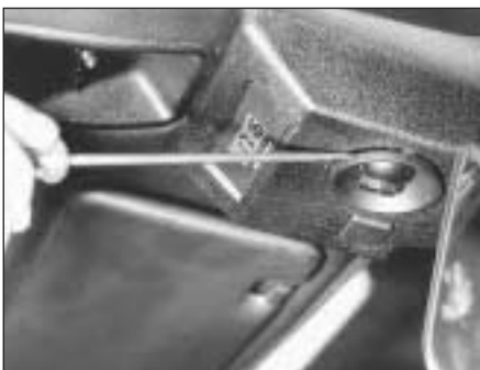
15.82 Roof-mounted clock retaining screw removal
