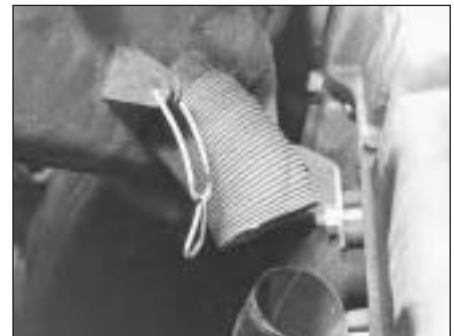
9A.5A Air cleaner hot air intake and lower retaining clip on the 999 cc model
