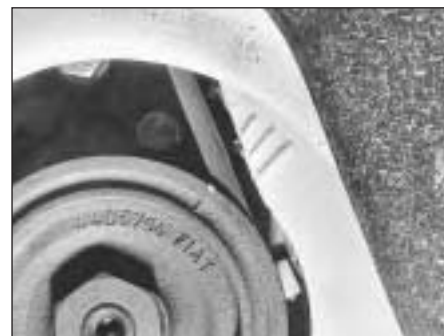
4.4 Ignition timing marks on belt cover
