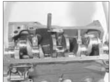
42.3 Lowering crankshaft into position
