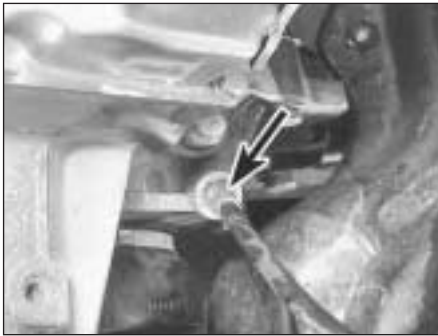
23.3 Speedometer cable connector at transmission
