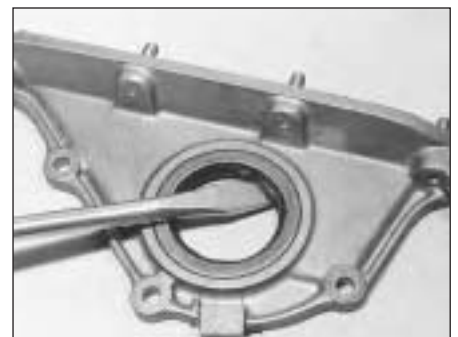
42.7A Removing oil seal from carrier
