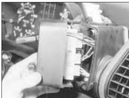
13.5A Withdrawing switch panel
