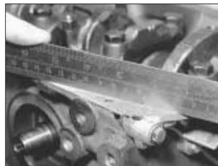
7B.141B . . . ensuring it is flush with the face of the cylinder block
