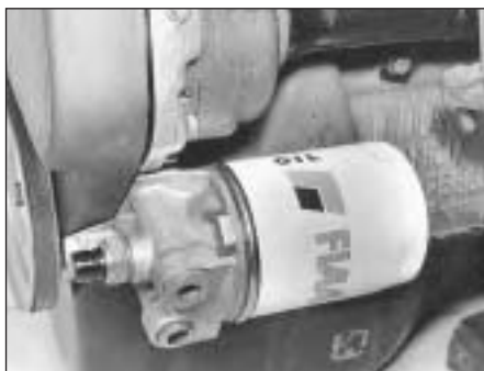
5D.29 Oil filter cartridge and mounting base
