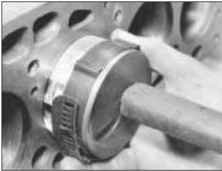
32.14 Fitting piston into cylinder bore
