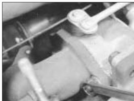
9F.16B Unscrewing turbocharger-to-exhaust manifold nut
