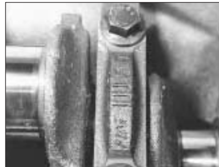
5C.66 Main bearing cap markings
