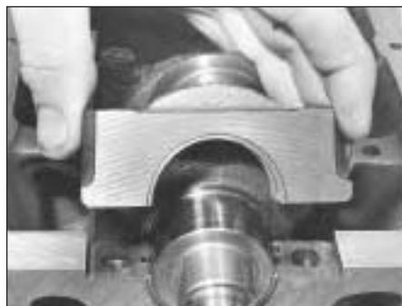
5D.6 Fitting a main bearing cap
