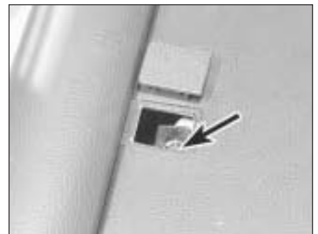
12.9 Heater upper fixing screw
