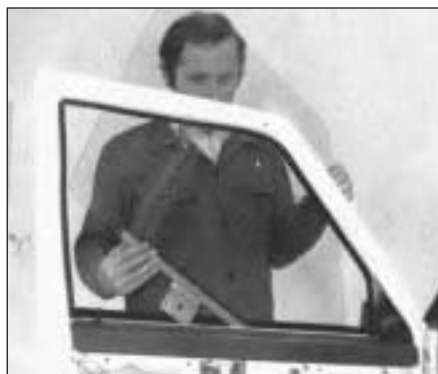
Fig. 12.8 Removing door glass (Sec 12)
