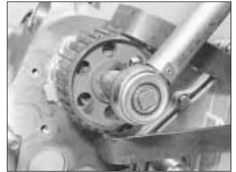
42.11 Tightening camshaft sprocket bolt. Note sprocket locking device
