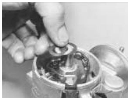
2.22B Washers above contact breaker
