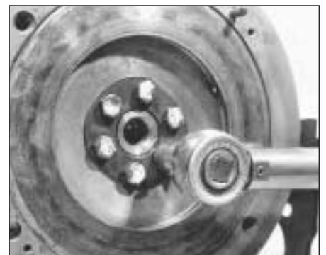
20.14 Tightening flywheel bolts
