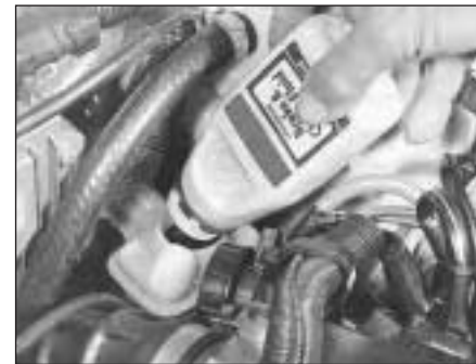
14B.14 Topping up the brake fluid reservoir (1301 cc Turbo ie model)
