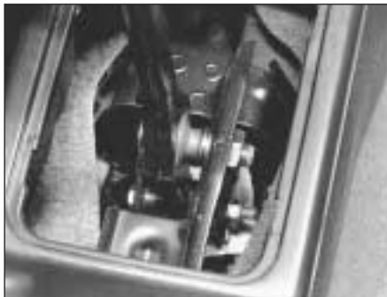
12B.15A Gear lever connection to the main connecting rod on the 1372 cc engine
