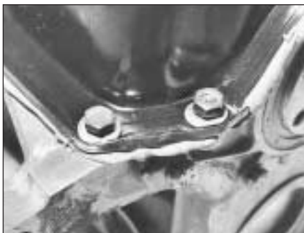
5B.63B Sump pan flange end fixing screw and nut
