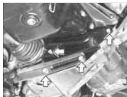
Fig. 13.19 Unscrew the bolts at the points indicated to release the gear linkage mounting bracket - 1372 cc ie and Turbo ie engines (Sec 7B)
