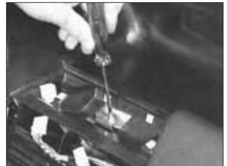
Fig. 13.31 Removing the heater unit-to-facia upper retaining screw (Sec 8D)
