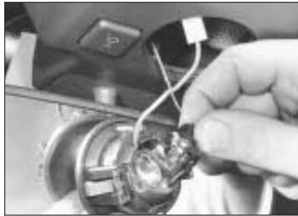
15.80B Roof-mounted spotlamp bulb removal
