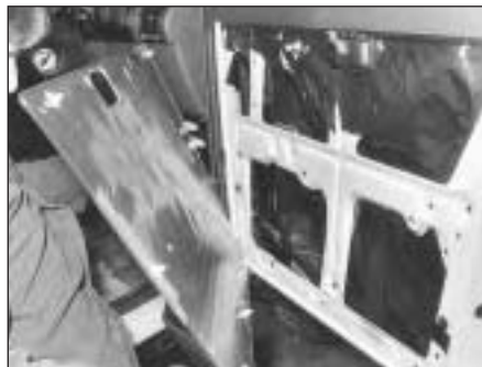
11.6 Removing door trim panel
