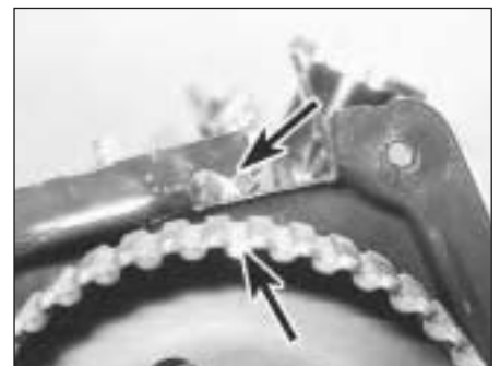
28.4 Camshaft sprocket alignment marks
