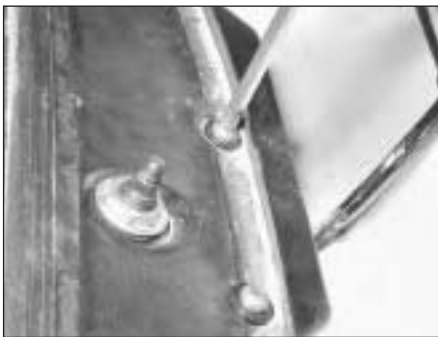
25.4 Removing windscreen wiper motor mounting screws
