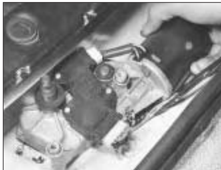
25.5B Removing windscreen wiper motor
