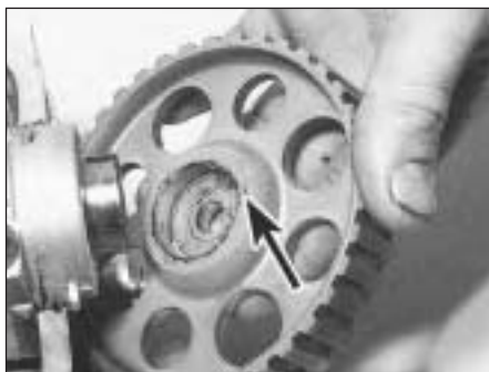
5B.22C Camshaft sprocket showing integral key (arrowed)
