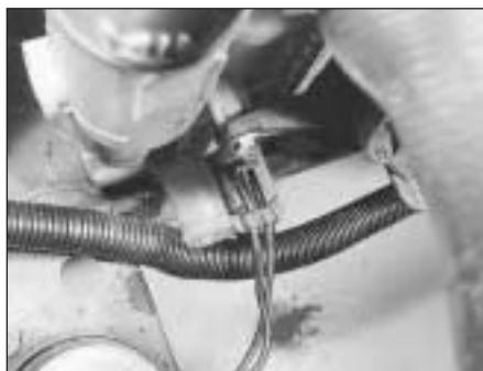
5C.19C Radiator fan cut-out thermostatic switch
