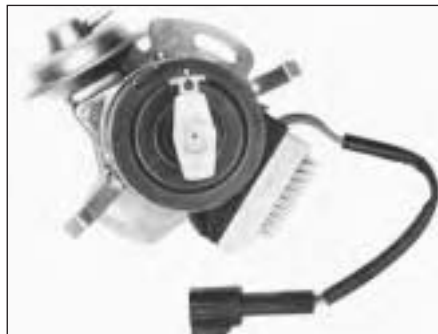
Fig. 13.72 Rotor aligned with arrow on distributor dust shield - 999 and 1108 cc engines (Sec 10)
