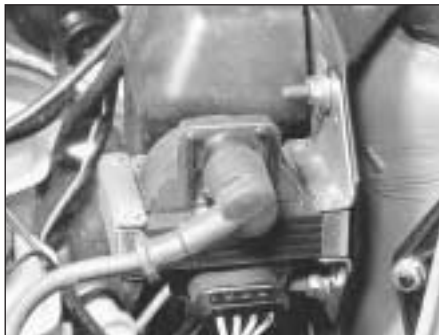
10.65 Ignition coil and connections on the 1372 cc ie engine
