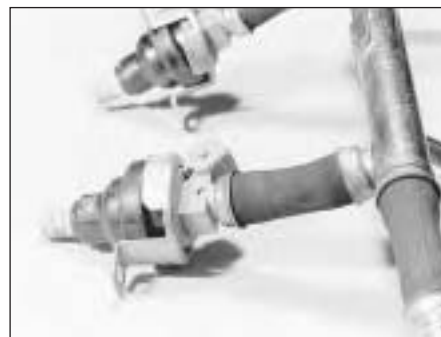
9C.81A Fuel injectors attached to fuel rail
