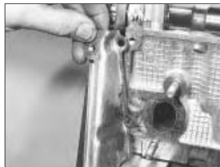
5D.20 Fitting the timing belt rear cover
