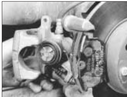
14B.26 Withdrawing the rear brake caliper
