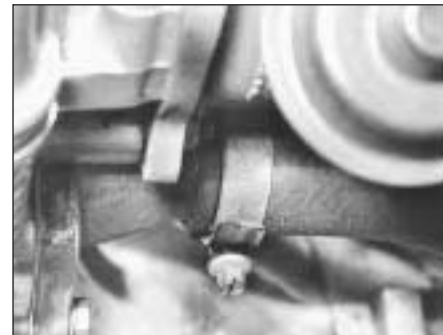
5C.7B Radiator hose at thermostat housing
