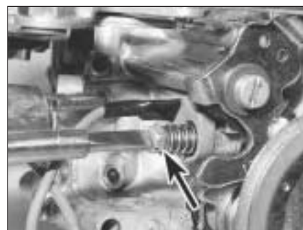
9B.36A Showing idle speed screw (arrowed) and . . .
