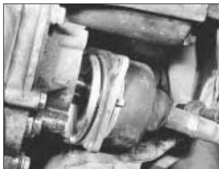
5C.25B Driveshaft joint garter withdrawn
