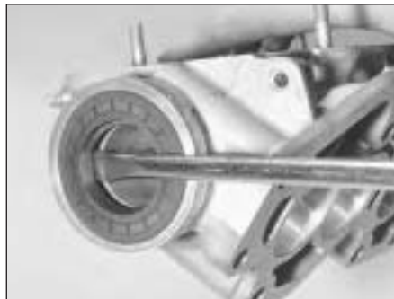
7B.97A Prising out the camshaft front oil seal
