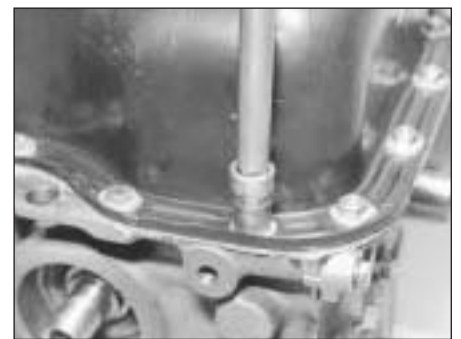
42.14 Tightening sump pan bolt
