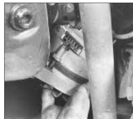
15.4 Removing the alternator from the 999 cc engine
