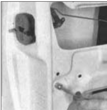
Fig. 12.12 Extracting glass guide channel screw (Sec 12)
