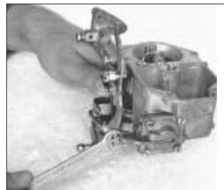
Fig. 3.17 Adjusting accelerator pump rod (Solex C32 DISA 11) (Sec 10)
