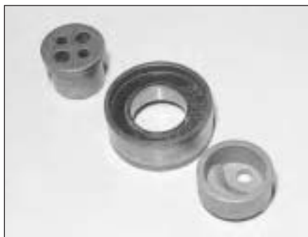
7B.38B The three sections of the timing belt tensioner
