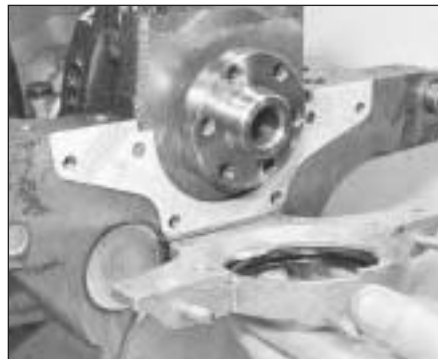
20.11A Crankshaft rear oil seal carrier and gasket
