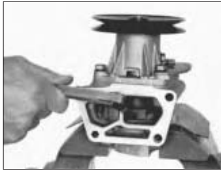
Fig. 2.6 Checking impeller clearance (Sec 9)
