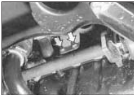
Fig. 13.66 Turbocharger mounting bracket bolts (arrowed) (Sec 9F)
