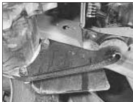
5C.31B Left-hand engine mounting and bracket
