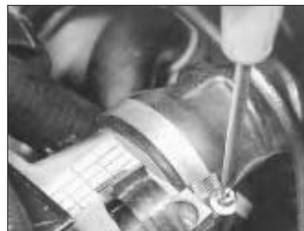
9C.57 Air outlet duct securing clip removal from airflow meter
