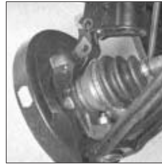
Fig. 1.18 Hub carrier detached from strut clamp (Sec 13)
