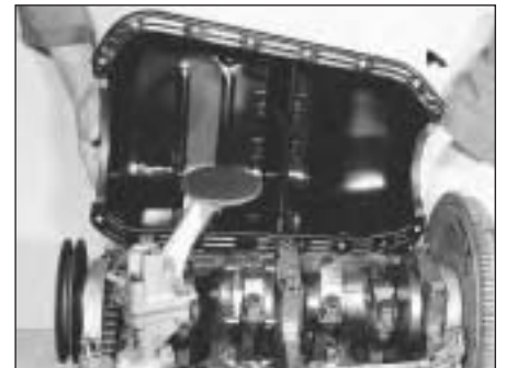
8.7A Fitting the sump pan
