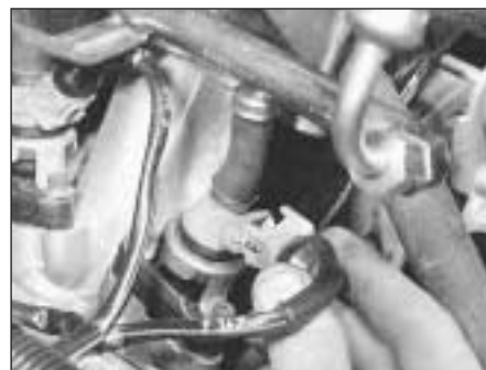
9C.81C Injector wiring plug refitting
