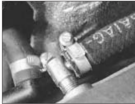
9C.70A Brake servo vacuum hose connection to inlet manifold
