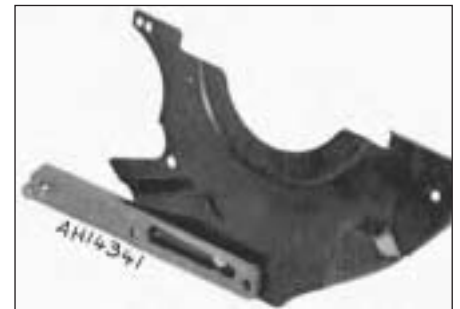
Fig. 1.20 Flywheel housing cover plate removed (Sec 13)
