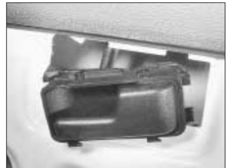
11.3B Remote control handle withdrawn
