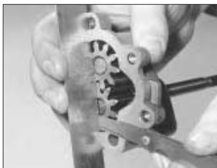
7B.177 Checking the gear endfloat
