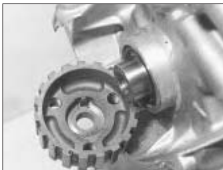
5D.16A Crankshaft sprocket showing integral key
