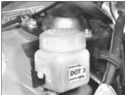
11.7A Clutch hydraulic fluid reservoir showing MIN and MAX markings
