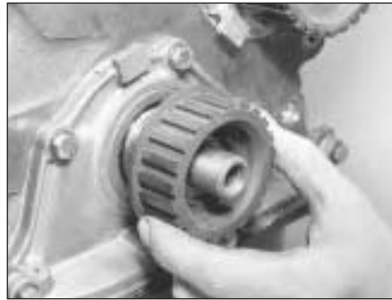
42.20 Fitting crankshaft timing belt sprocket
