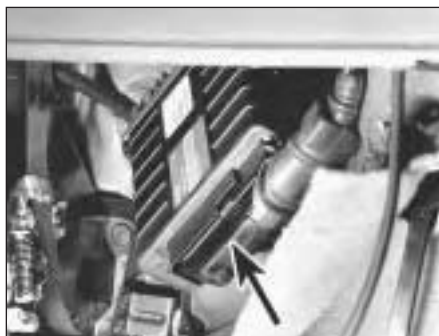
9D.58A Detach the multiplug (arrowed) . . .
