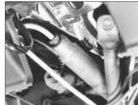
11.12 Clutch master cylinder and hydraulic pipe connections
