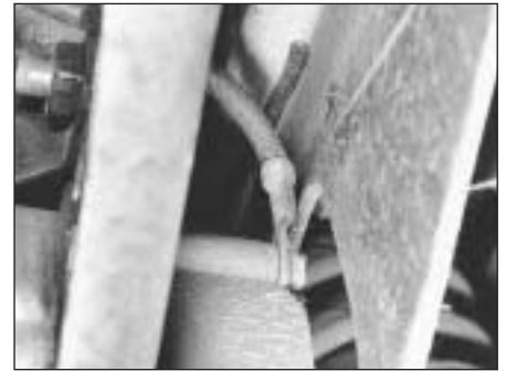
7C.33 Disconnect the transmission earth strap
