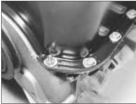
8.7B Sump pan nut, bolts and washers
