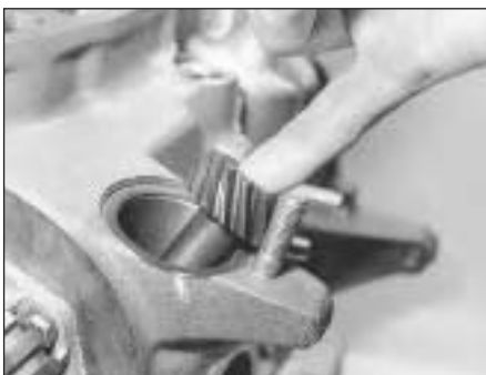
42.15 Fitting oil pump driveshaft
