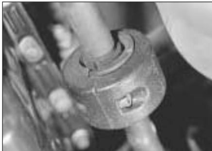
13.24 Right-hand driveshaft damper weight
