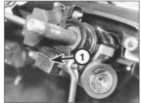
11.4 Unscrewing steering column switch clamp nut
