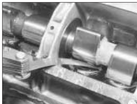
25.4 Checking a valve clearance
