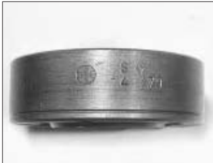
13.21 Outer track reference groove
