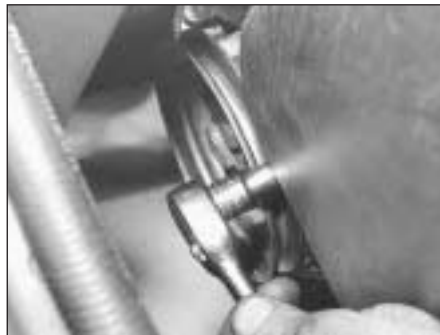
5B.6 Timing cover lower fixing bolt removal
