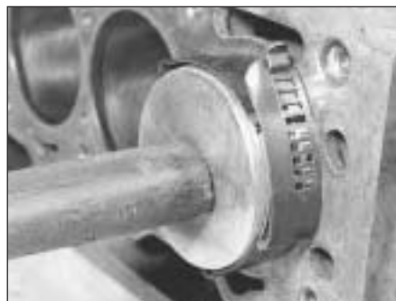
9.19 Fitting a piston/connecting rod
