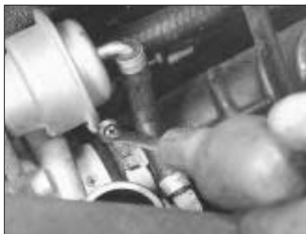
9F.17 Releasing turbocharger air hose clip
