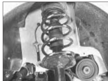
3.5 Withdrawing a front strut
