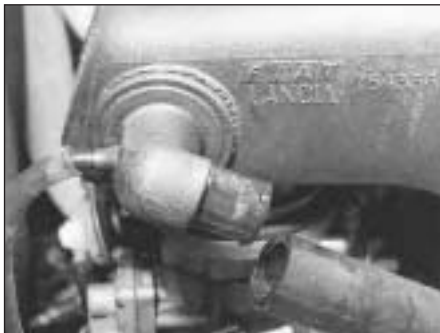
9A.5C Air cleaner breather hoses on the 999 cc model
