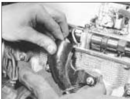
5D.32 Air cleaner hot air collector plate
