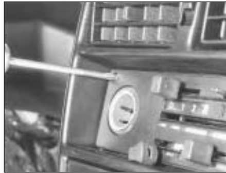
12.6A Heater control panel screw
