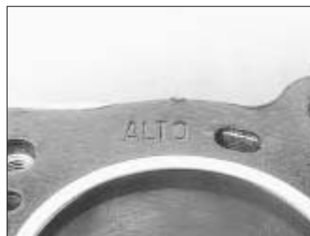
5B.50B Cylinder head gasket top surface marking
