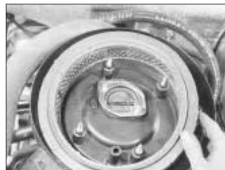
2.6 Removing air cleaner element
