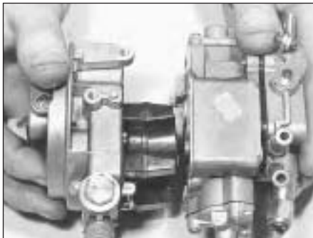
9B.26F Main parts of the Weber 32 TLF carburettor
