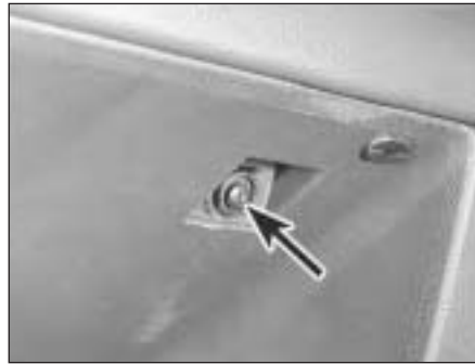
22.5A Fascia fixing screw inside glovebox
