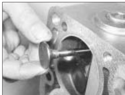
17.17B Inserting a valve into its guide
