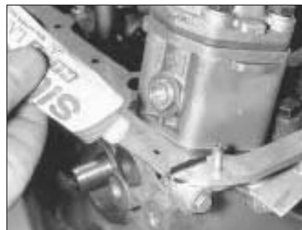
7B.165 Apply sealant to the front oil seal housing/cylinder block joint
