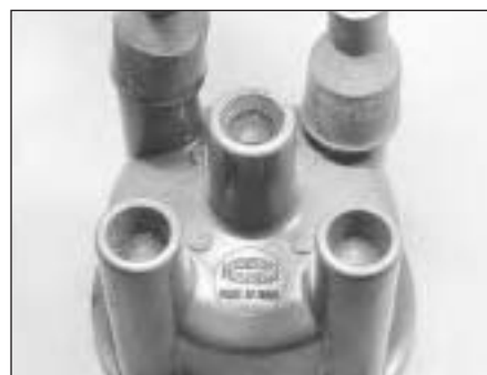
11.7 Distributor cap HT lead markings
