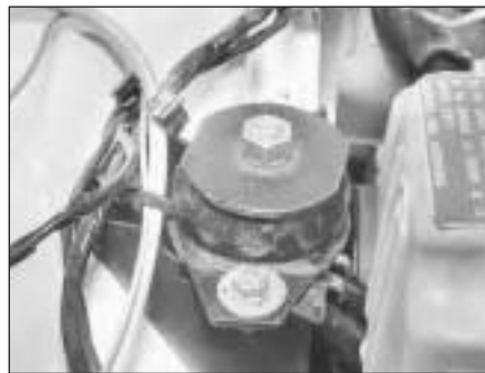
44.8D Right-hand mounting bolted up
