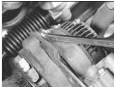
8C.53 Tightening the alternator adjuster nut
