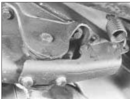
10.4 Pressure regulating valve bracket and tension spring
