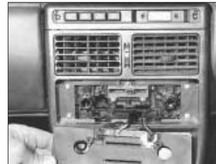
15.69B . . . and withdraw the heater control panel
