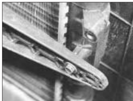
8C.22 Cooling fan to radiator securing bolt
