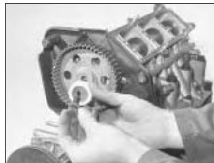
7B.41 Removing the crankshaft sprocket bolt, plain washer and thrust washer
