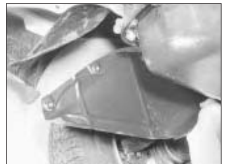
44.32 Inner wing protective shield
