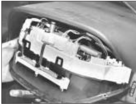
15.59A . . . withdraw the instrument panel . . .
