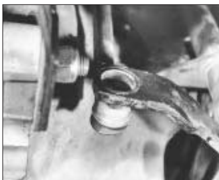
5C.24B Gearchange rod with ball socket connection
