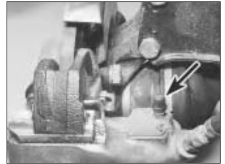
12.8 Caliper bleed screw with dust cap fitted
