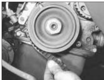
6B.19B Removing the timing belt
