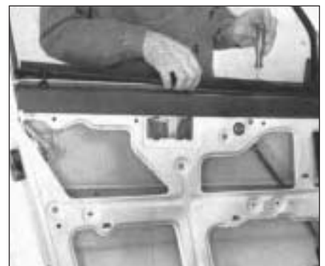
Fig. 12.7 Removing door weatherseal (Sec 12)
