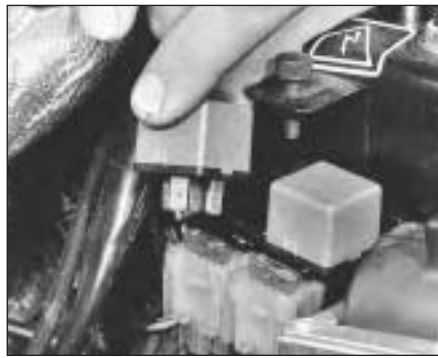
9D.27 Fuel pump relay removal
