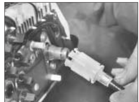
23.2 Speedometer cable connector at head
