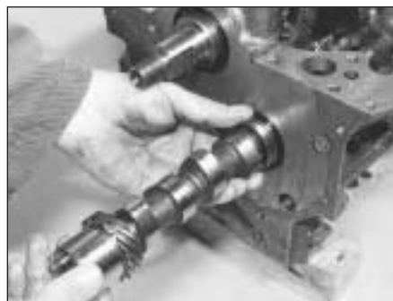
20.16A Fitting camshaft
