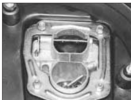
9A.9A Circular type air cleaner fixing nuts
