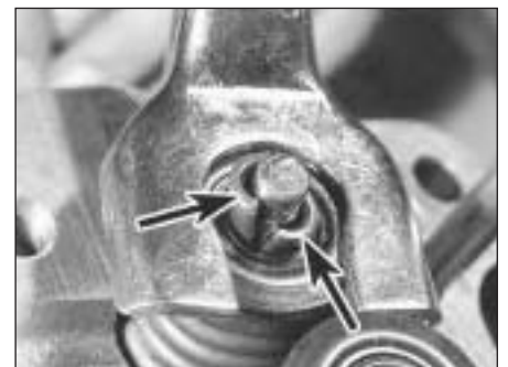
17.19 Fitting split collets
