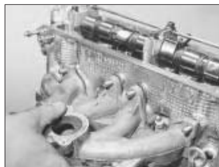
5D.25B Fitting the inlet manifold
