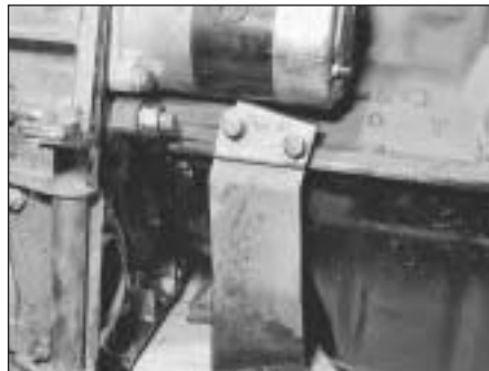
5C.60B Exhaust pipe support bracket attached to crankcase
