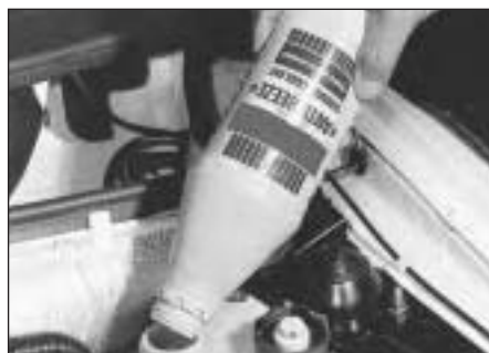
8B.4 Topping up the expansion tank with antifreeze on the 1301 cc engine
