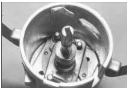
7.13 Marelli distributor centrifugal weights and springs
