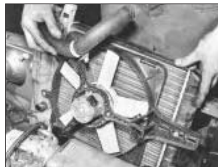
5C.19D Removing the radiator/fan assembly
