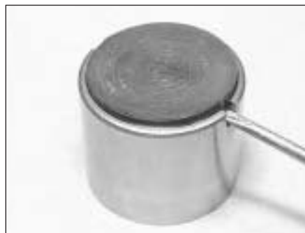
26.2 Removing a shim from a cam follower
