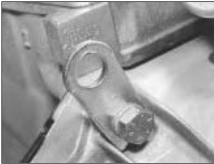
44.2 Lifting lug at bellhousing bolt
