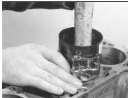
7B.194B Tapping a piston into its bore
