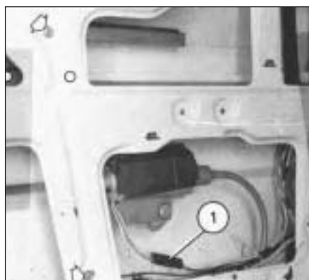
Fig. 9.11 Power-operated window motor (Sec 31)
