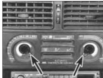
15.69A . . . undo the retaining screws (arrowed)
