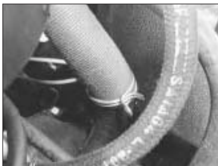
2.1 Air cleaner hot air intake
