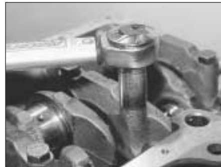
7DS.14 Tighten the main bearing cap bolts to the specified torque setting
