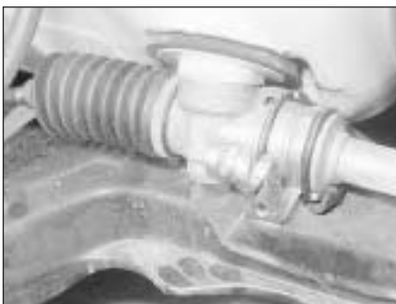
6.4 Steering rack housing at pinion end
