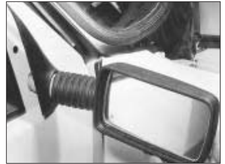
24.4 Withdrawing exterior mirror and trim plate
