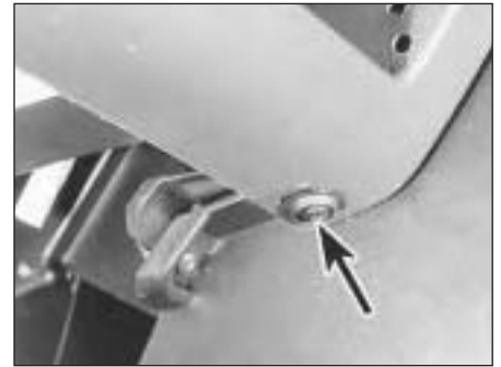
22.5B Fascia panel lower mounting screw at centre console
