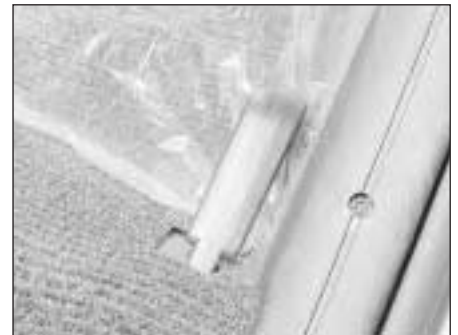
14.7 Tailgate remote control release lever
