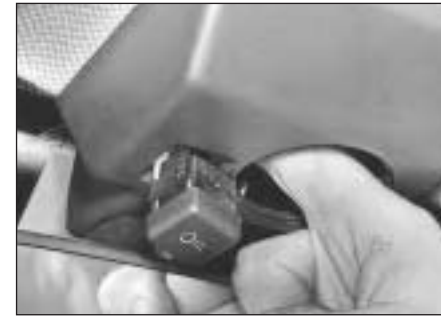
15.81 Roof-mounted spotlamp switch removal
