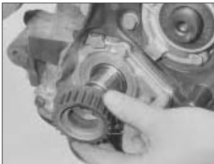
7B.47 Refitting the crankshaft sprocket
