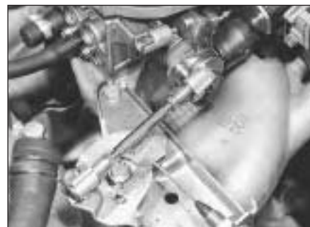
9D.22 Accelerator control rod and cable connections
