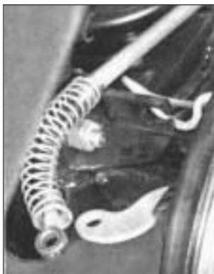
Fig. 11.11 Handbrake cable and lever at brake backplate (Sec 11)
