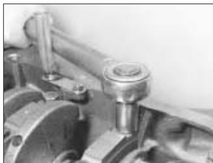
42.4B Tightening a main bearing cap bolt
