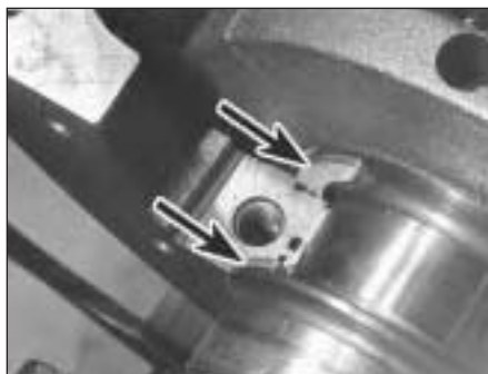
7D.7B . . . sliding them into position each side of the No. 5 main bearing
