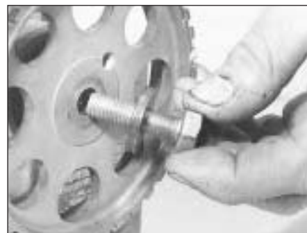
5B.22B Camshaft sprocket bolt and washer
