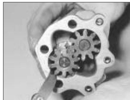
7B.176 Check gear-to-body clearance
