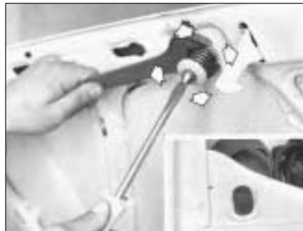
Fig. 12.2 Adjusting bonnet lock striker (Sec 8)
