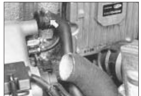
Fig. 13.56 Disconnecting the injector air cooling hoses and the supplementary air valve hose on the 1372 cc Turbo ie engine (Sec 9E)
