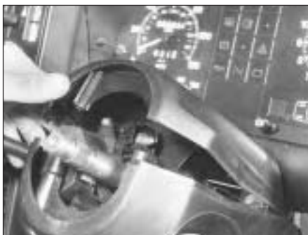
5.2 Removing steering column shrouds
