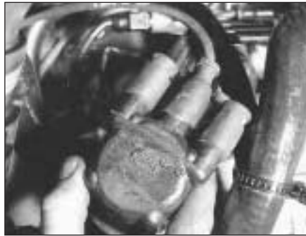
10.38 Removing the distributor cap
