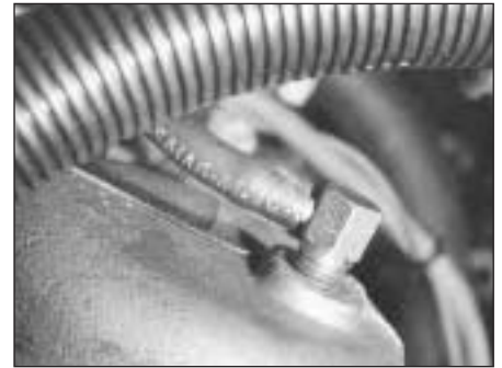
9C.70B Fuel pressure regulator vacuum hose connection at the inlet manifold
