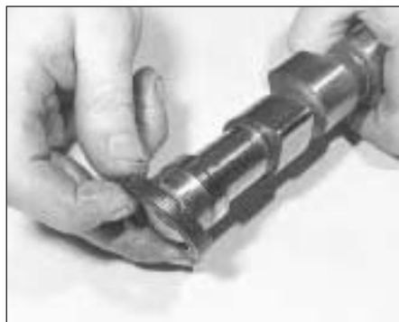
5B.26A Camshaft oil seal
