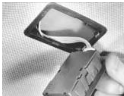
15.86 Remote control receiver unit removal
