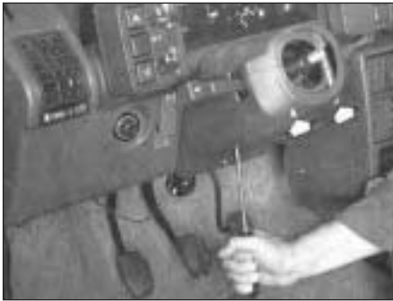
Fig. 10.2 Removing steering column shroud screws (Sec 5)
