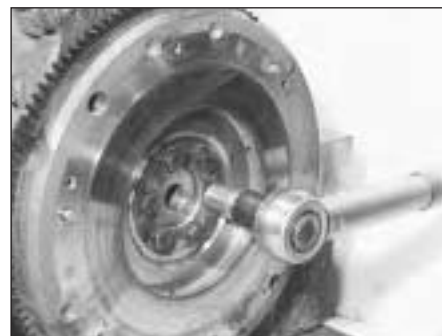
5D.14 Tightening a flywheel bolt
