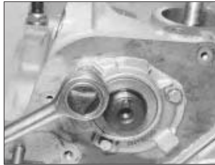
42.10B Tightening auxiliary shaft end plate bolt
