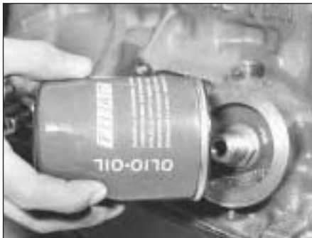
2.8 Screwing on the oil filter (903 cc)
