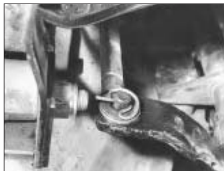
5C.24A Gearchange rod connecting pin and spring clip
