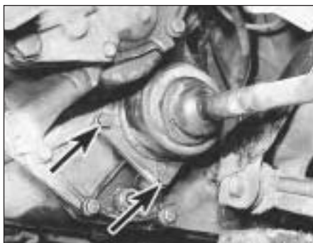
5C.25A Two of the left-hand driveshaft joint garter retaining plate screws (arrowed)
