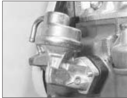
3.6A Fuel pump on mounting studs
