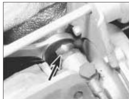
9F.18A Releasing turbocharger coolant inlet union (arrowed)
