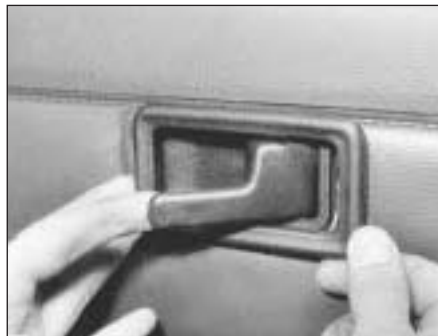
11.3A Removing remote control handle escutcheon
