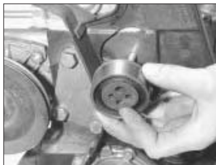
7B.38A Timing belt tensioner removal
