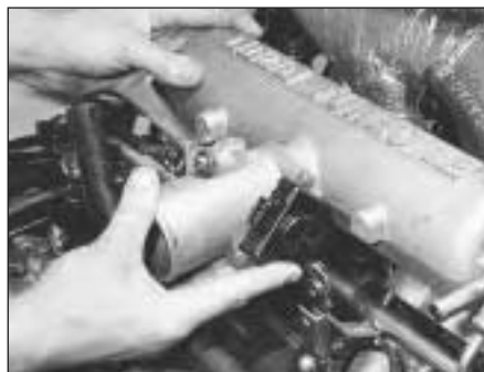
9C.73 Removing the inlet manifold
