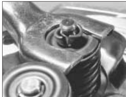
39.2 Valve spring compressor and split collets
