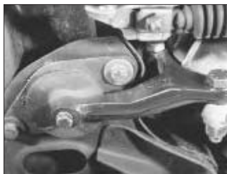
6B.16A Engine/transmission centre mounting
