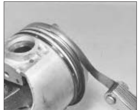
18.24A Checking piston ring groove clearance
