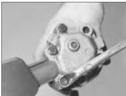
7B.171 Undo the oil pump cover bolts
