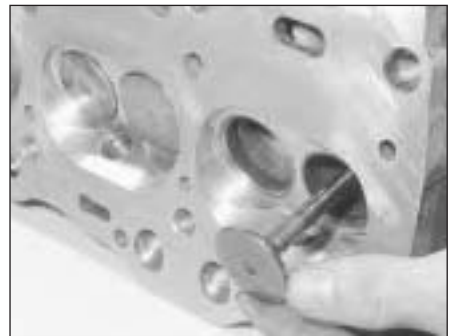
7B.130B Valve assembly - 1372 cc engine; insert valve into guide . . .
