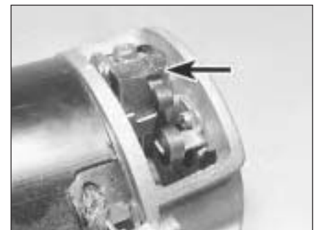
9.4 Starter motor brush partly withdrawn
