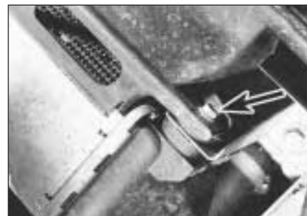
9F.43 Intercooler mounting bolt (arrowed) on 1301 cc engine
