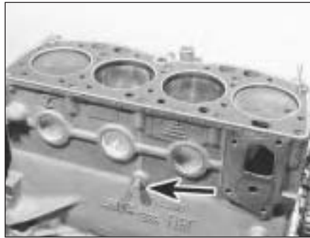
29.21B Cylinder head gasket in position - cylinder block drain plug arrowed
