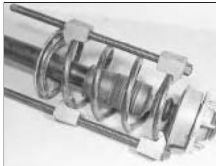
3.6 Spring clamps in position
