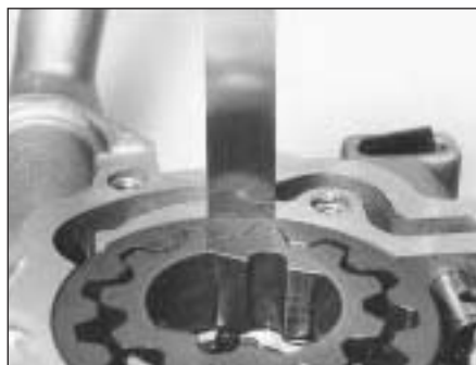
5B.74A Checking the oil pump gear-to-housing clearance
