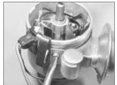
2.21 Extracting vacuum diaphragm unit screw
