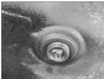
7A.12A Engine sump drain plug - 1372 cc engine
