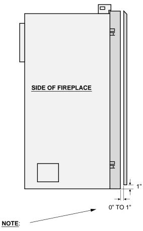
This face has an adjustable bracket that allows for different facing depths to be tucked under the face.
