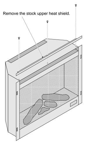
Place the upper heat shield included with this kit on top of the fireplace (note position of heat shield). Place the stock heat shield on top of it and secure with the same screws.
