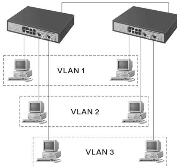
Fig. 2-6 Attribute-based VLAN Diagram
