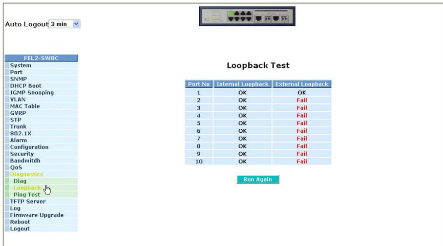
The screenshot shows the web interface of the switch. On the left is a navigation menu with categories like System, Port, and Diagnostics. The 'Loopback' option under Diagnostics is highlighted. The main content area is titled 'Loopback Test' and contains a table with the following data:
