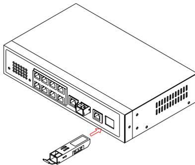
Fig. 2-1 Installation of Optional SFP Fiber Transceiver
