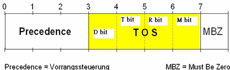
DiffServ DSCP Priority act on DSCP field of IP Header. In the late 1990s, the IETF redefined the meaning of the 8-bit SERVICE TYPE field to accommodate a set of differentiated services (DS). Under the differentiated services interpretation, the first six bits comprise a codepoint, which is sometimes abbreviated DSCP, and the last two bits are left unused.
