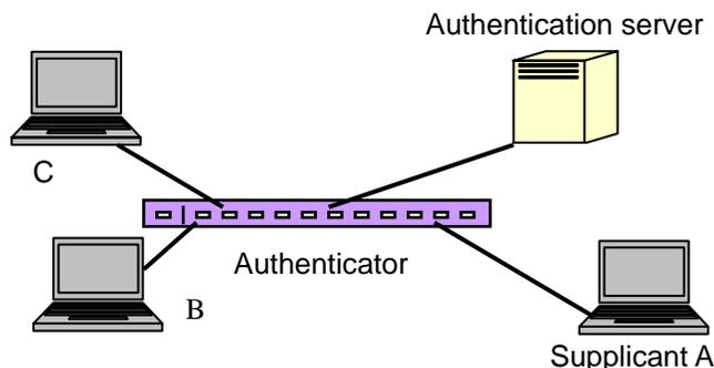
The Fig. 3-43 shows the procedure of 802.1x authentication. There are steps for the login based on 802.1x port access control management. The protocol used in the right side is EAPOL and the left side is EAP.
