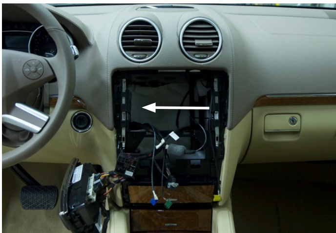
7) Access EIS wiring through opening
