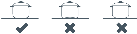
Fig. 16b Efficient and inefficient saucepan bottoms
