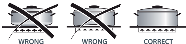
Inefficient and efficient saucepan bottoms
