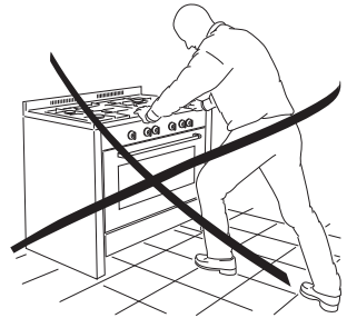
Fig. 10 Incorrectly moving the cooker
