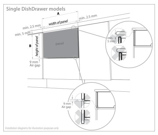
The following calculations assume the top of the panel is aligned with the top of the adjacent cabinetry:
