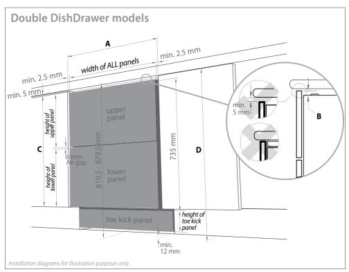
The following calculations assume the top of the upper panel is aligned with the top of the adjacent cabinetry. The final panel/cabinetry alignment is achieved by adjusting the feet:
