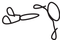
Wire clip (2) (for securing Drain hose joiner)
