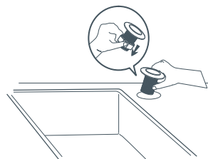
Fig. 12 Fitting the air switch
