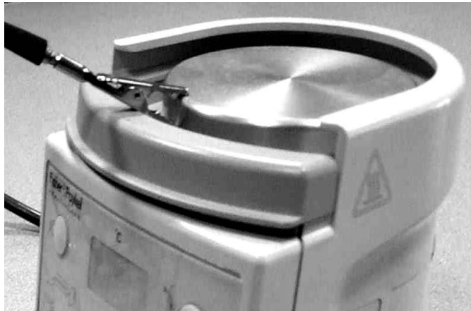
Figure 5.1 Showing the correct location of ground test point on the heater plate
