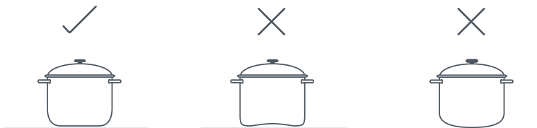
Fig.20 Efficient and inefficient pan bases
