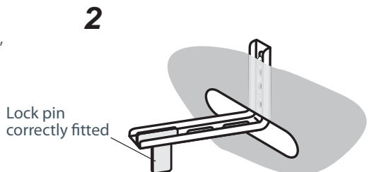
Fig. 10c Fitting the lock pin through the bracket
