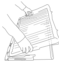
Fig.25 Removing lid from rear clips and side retainers
