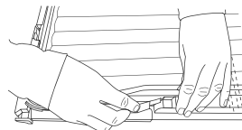
Fig.27 Fit lid under side retainers
