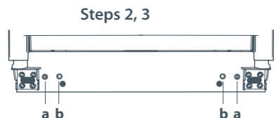
Fig.5 Levelling the refrigerator
