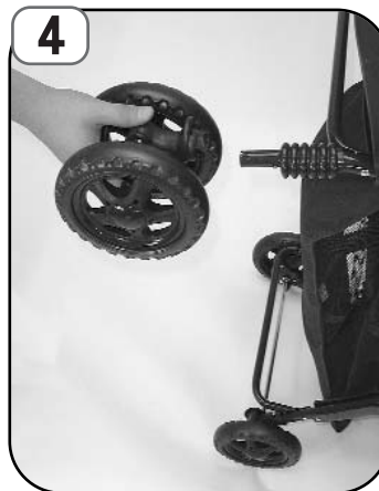
IMPORTANT! Lock wheel swivel into place before inserting wheel assembly (A). There is a right side assembly for the right side of the stroller. Fit a front wheel assembly to each front leg. Push assembly firmly onto each leg so that the buttons "snap" into the holes in the wheel brackets.
