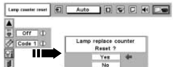
Move the pointer to Lamp counter reset and then press SELECT button. The message "Lamp replace counter reset?"
